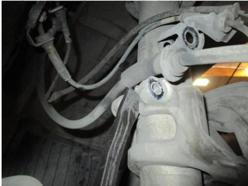
6. Using a 13 mm socket, remove the (3) bolts that hold the strut housing into the vehicle. Be careful to use a helper to hold the strut from the bottom of the car. If the vehicle is equipped with EDC shocks, you will need to disconnect the plug from the top of the strut.
