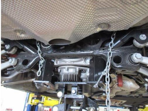
10. To remove the OEM Sway bar from the vehicle, you must first slide the passenger side towards the rear of the vehicle. This will allow you to rotate the left side sway bar arm above the control arm. Once above the arm you can rotate the bar until it slides out through the drivers side of the vehicle.
