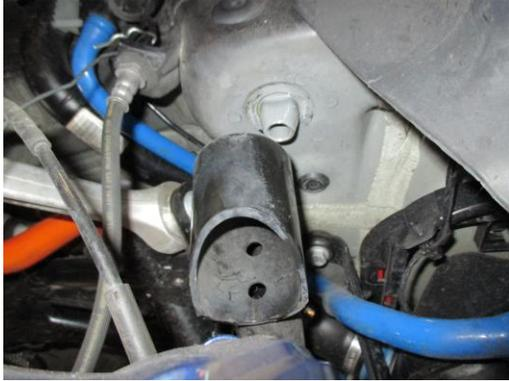
5. Reinstall the OEM reinforcement bar, and reinstall the splash guards.
