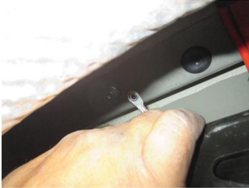
7. Using a 18 mm socket, remove the rear brake calipers, and hang them out of the way. Be careful not to damage or kink any lines. Using a 16 mm wrench, remove the nuts, from the factory end links.
