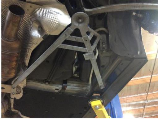
6. Release the plastic clips from the subframe so the wire harness can have room to move freely. Remove the ground wire from the chassis by removing the 10 mm nut.
