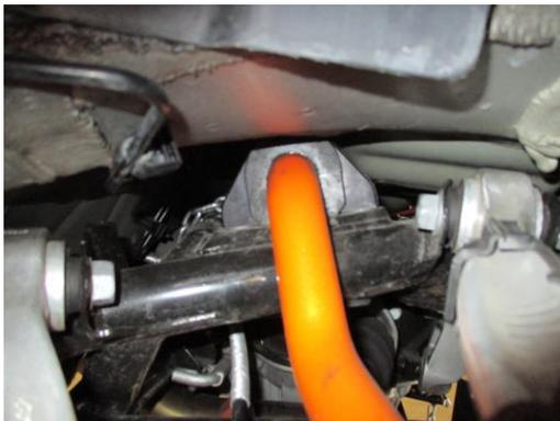
4. Raise the sub-frame back into position. The front mounts have positioning pins, for alignment. Be careful not to pinch any lines, or wires. Torque the sub frame bolts to 65 lb-ft. Reattach the calipers, and torque to factory specs.
