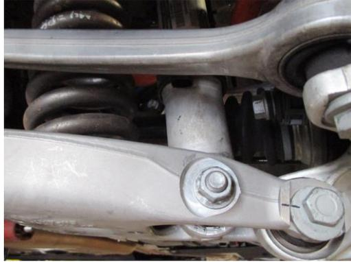
9. The next step will require the drop of the rear sub frame, it is important to make sure you have slack in both the ABS, and ride height sensor wires as the sub frame comes down. Slowly lower the sub frame just enough to get a E12 socket on the OEM bushing brackets. (approximately 2") Remove the (4) bolts attaching the sway bar bushings.
