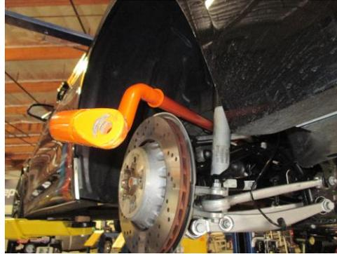
2. It is important to make sure the sway bar is positioned under the upper control arm on the passenger side when sliding bar into place. The correct orientation would put the bar under both the drivers, and passenger upper control arms.
