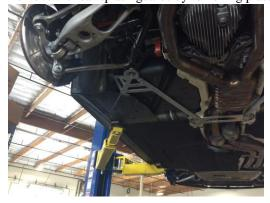
5. Using a T60 torx socket, a T40 torx socket, and a 16mm socket, remove the bolts that hold the rear chassis reinforcement to the body.
