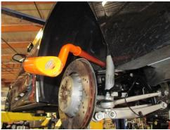
2. It is important to make sure the sway bar is positioned under the upper control arm on the passenger side when sliding bar into place. The correct orientation would put the bar under both the drivers, and passenger upper control arms.
