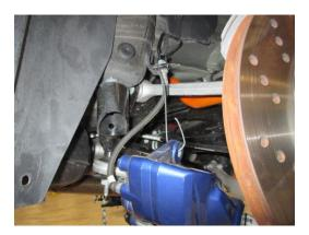
8. Using either a floor jack, or a trans jack, support the rear differential. Remove the rear shock mount bolts. Next remove the (4) 15mm sub frame bolts.
