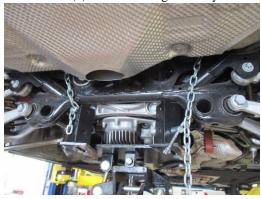
10. To remove the OEM Sway bar from the vehicle, you must first slide the passenger side towards the rear of the vehicle. This will allow you to rotate the left side sway bar arm above the control arm. Once above the arm you can rotate the bar until it slides out through the drivers side of the vehicle.
