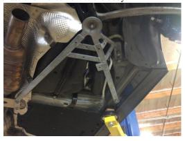
6. Release the plastic clips from the subframe so the wire harness can have room to move freely. Remove the ground wire from the chassis by removing the 10 mm nut.
