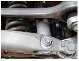
9. The next step will require the drop of the rear sub frame, it is important to make sure you have slack in both the ABS, and ride height sensor wires as the sub frame comes down. Slowly lower the sub frame just enough to get a E12 socket on the OEM bushing brackets. (approximately 2") Remove the (4) bolts attaching the sway bar bushings.
