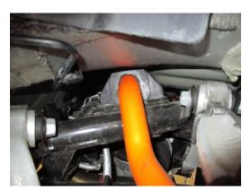
4. Raise the sub-frame back into position. The front mounts have positioning pins, for alignment. Be careful not to pinch any lines, or wires. Torque the sub frame bolts to 65 lb-ft. Reattach the calipers, and torque to factory specs.
