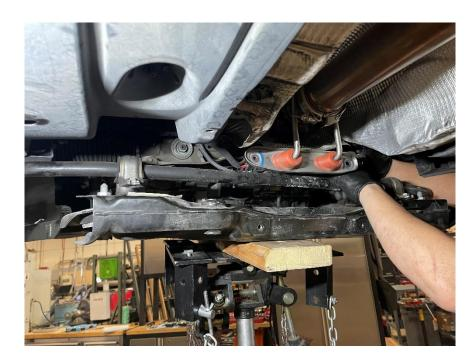
15F As you lower the subframe you will gain access to this line clip. Unclip this attachment point on driver side near the forward subframe mount.
