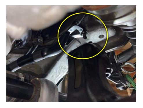
16F Lay out the factory sway bar with the aFe Control sway bar to match the orientation.
