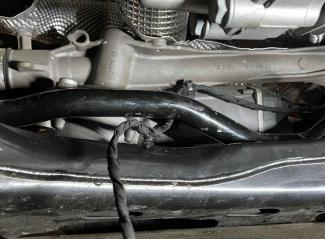
Route this wire harness up and around the factory sway bar so it rests on top of the sway bar. This will keep the wire harness out of harms way when the sway bar is removed towards the rear of the vehicle.
