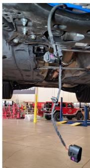
Pry the push-clip to release sensor line from the subframe
