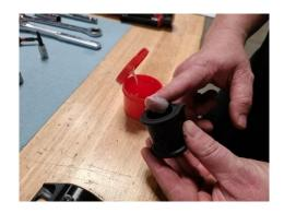
Install the bushing onto the sway bar. The bushings should be positioned just outside of the centering rings. Slide the aFe Control bushing bracket onto the bushing. The thin black aluminum spacer goes between the bushing and the subframe. Fully tighten this hardware to 40 ft lbs.
