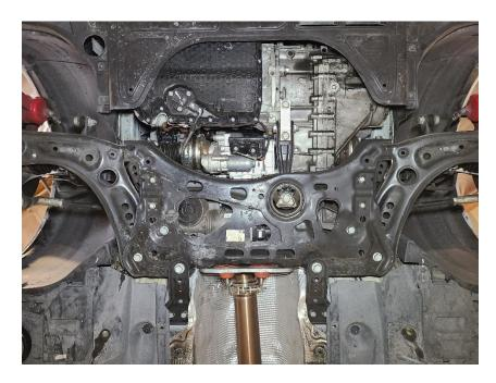
3F Disconnect the ride height sensor bracket from the driver side and passenger side lower control arm, using a 10mm socket.
