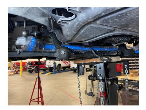
18F Grease the front bushings (5343) with the supplied silicone lube. Install bushing onto the sway bar. The bushings should be positioned just inside of the centering rings.
