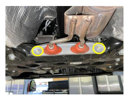
6F Disconnect the engine/trans dog bone mount with a 21mm wrench and socket.
