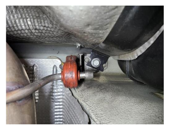
6R Remove exhaust hanger bolt from both sides with a (13mm socket).
