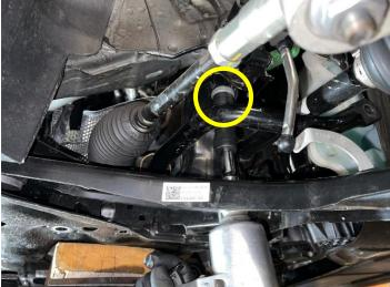
Lower the sub frame just enough so the sway bar can be removed towards the rear of the car. You will need to lift the steering rack and sneak the sway bar under and out the back.
