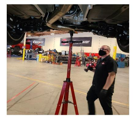
5R Unbolt the center brace and exhaust hanger with a (13mm socket).
