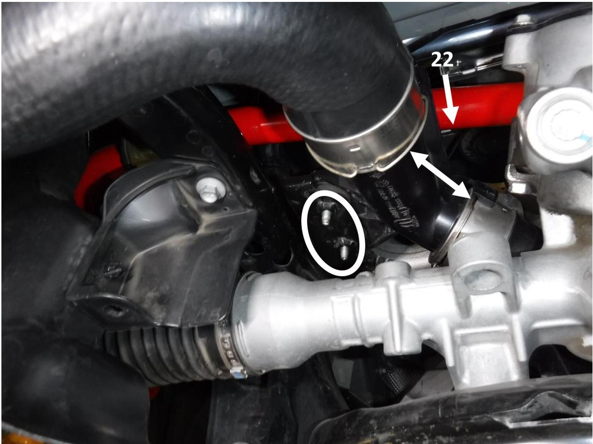
21. Disconnect both quick connect adapters from the cold side intercooler tube plastic adapter.
