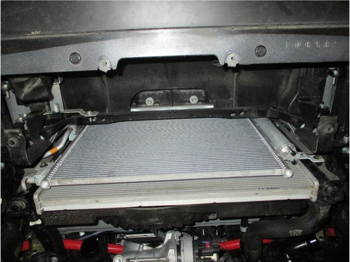
35. Remove the intercooler from the vehicle.
