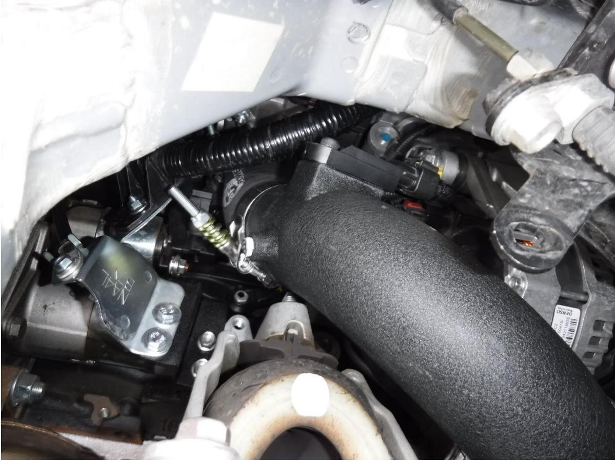
50. Install the supplied 2-1/4" x 2" x 45° coupling along with one (1) of the supplied 2-1/2" clamps onto the reduced end of the aFe upper cold side intercooler tube (do not tighten the clamp yet).
