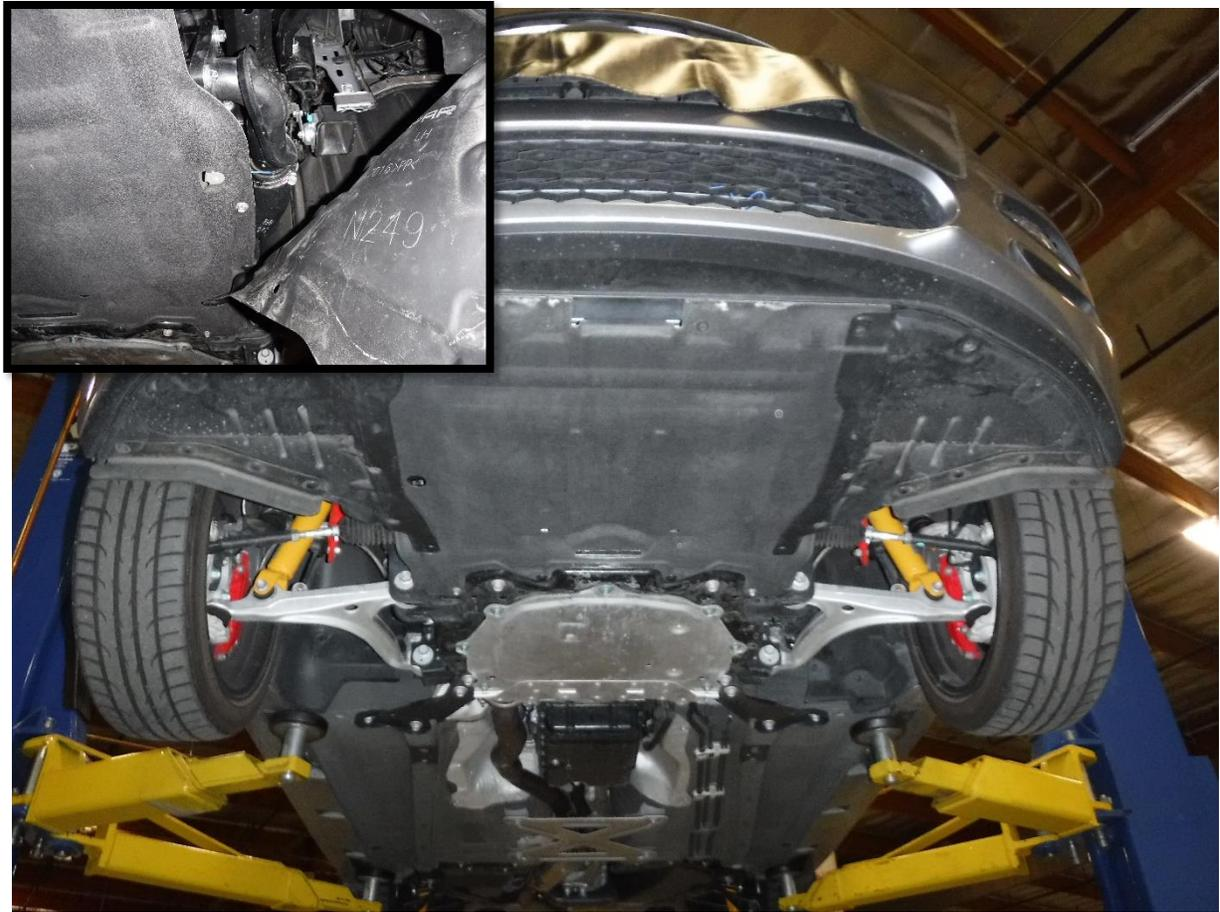
13. Remove all the screws and clips securing the belly pan to the vehicle.
