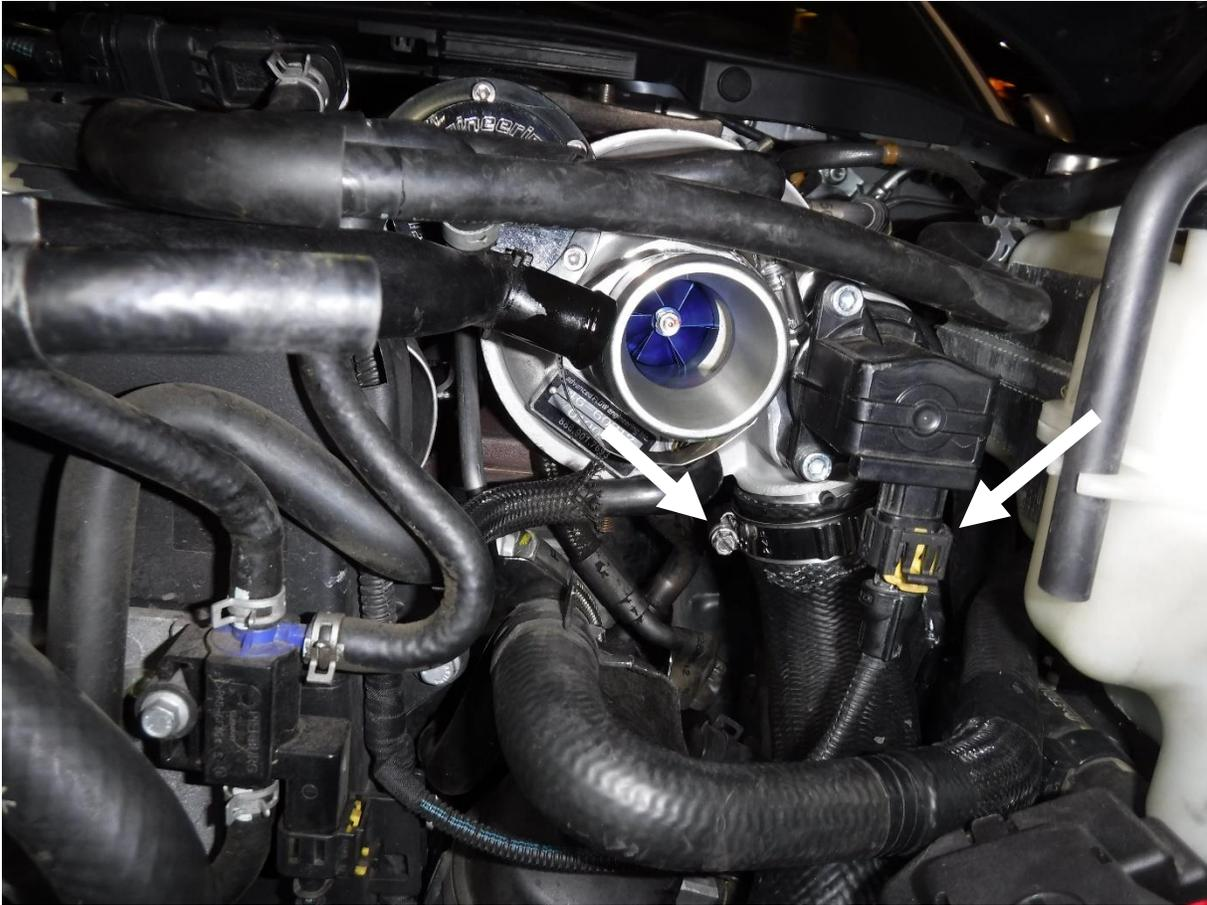
9. Disconnect recirculation valve connection by sliding the yellow locking tab back on the connector, on the front of the turbo, then press the black tab to pull the connections apart.
