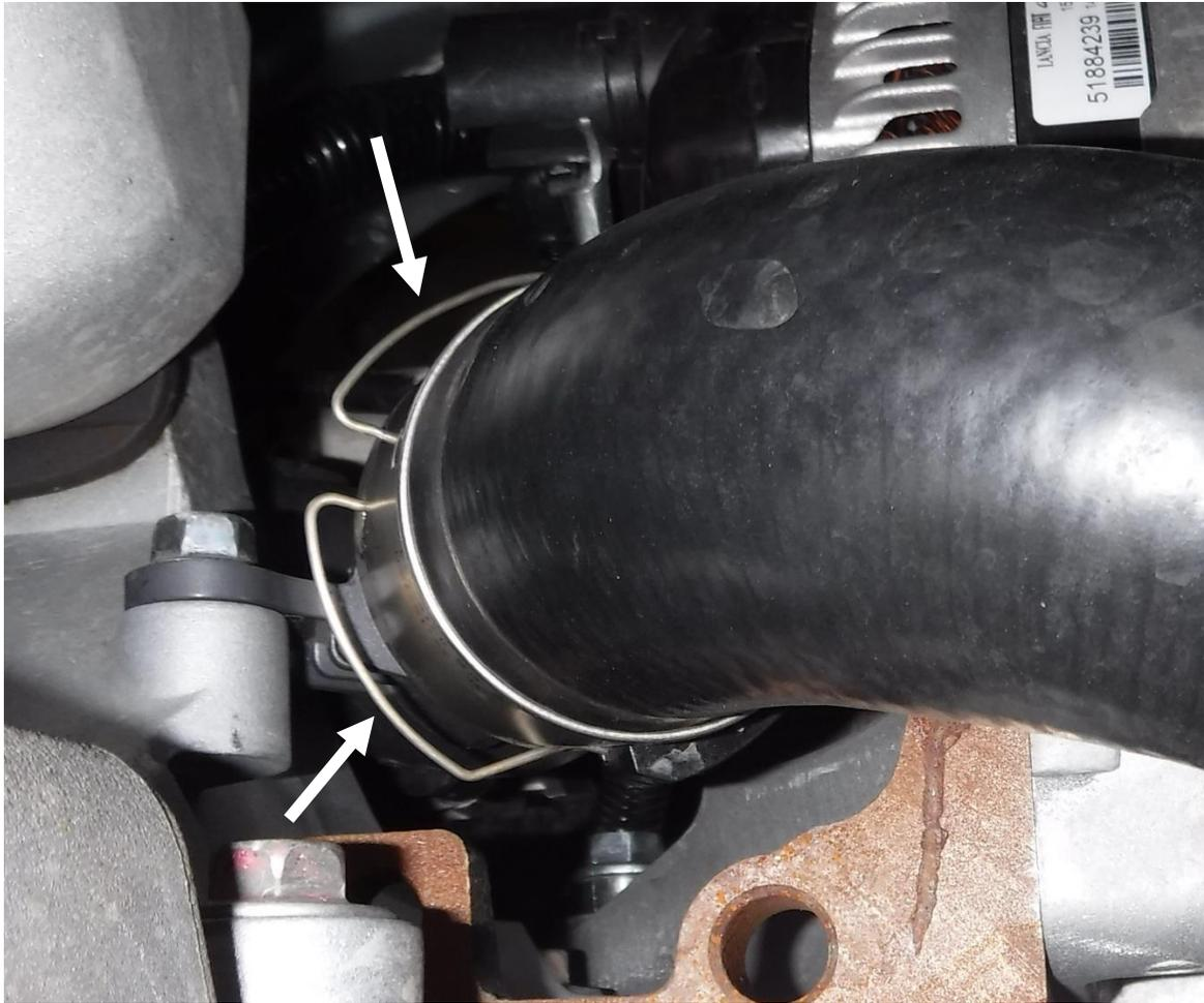
18. To disconnect the quick connect adapter you will need to lift both sides of the retaining clip that secure the intercooler tube to the plastic adapter using two flat head screwdrivers and pull the lower hot side intercooler tube off of the plastic adapter at the same time.
