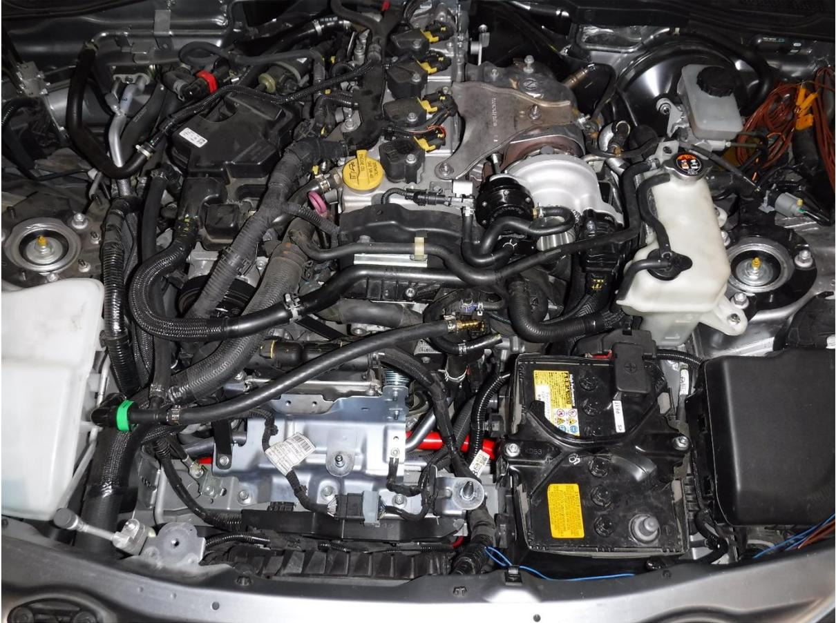
3. Disconnect all vacuum hoses from the air box and intake tube.
