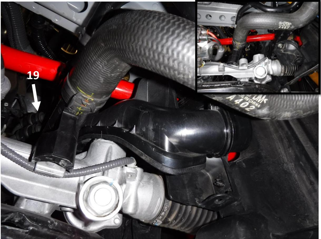
19. Remove the screw securing the lower radiator hose mounting bracket to the subframe so that it can be moved to the side.
