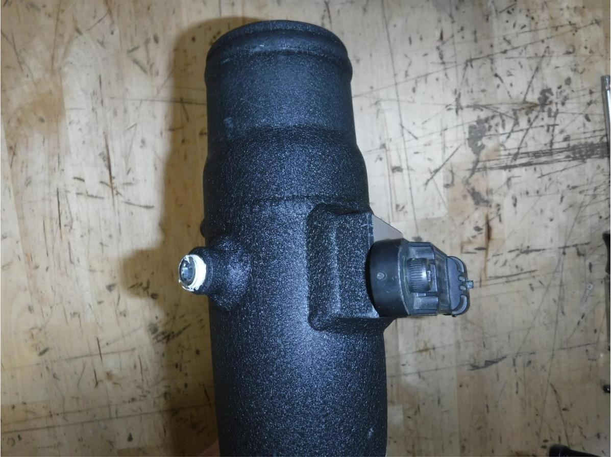
46. Remove the MAP sensor from the factory upper cold side intercooler tube.
