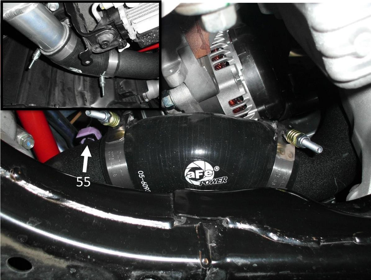
52. Install the supplied 2-1/2" x 45° coupling with one (1) of the supplied 2-7/8" clamps onto the aFe upper cold side intercooler tube.
