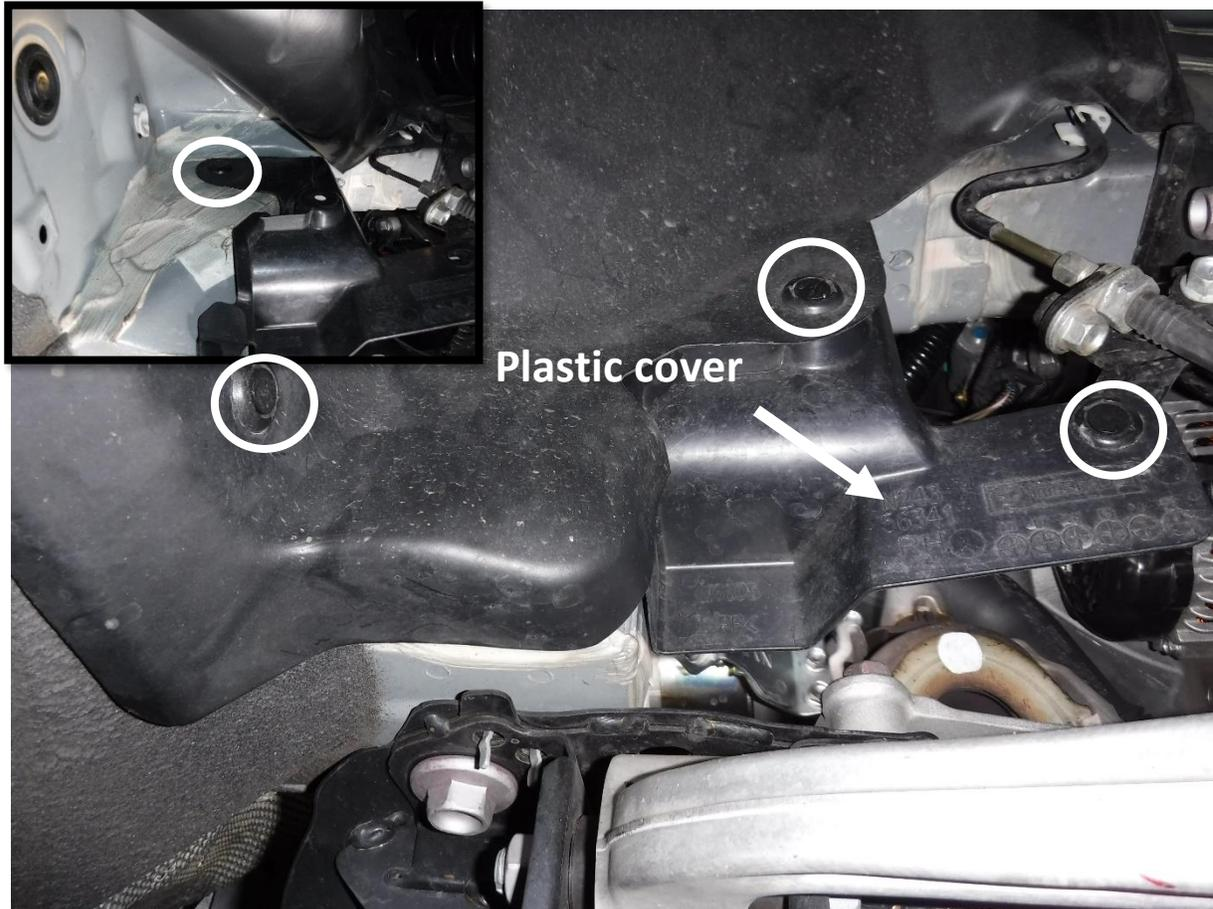
25. Behind the passenger side tire, remove the three (3) clips securing the plastic cover and the inner fender liner to the vehicle.
