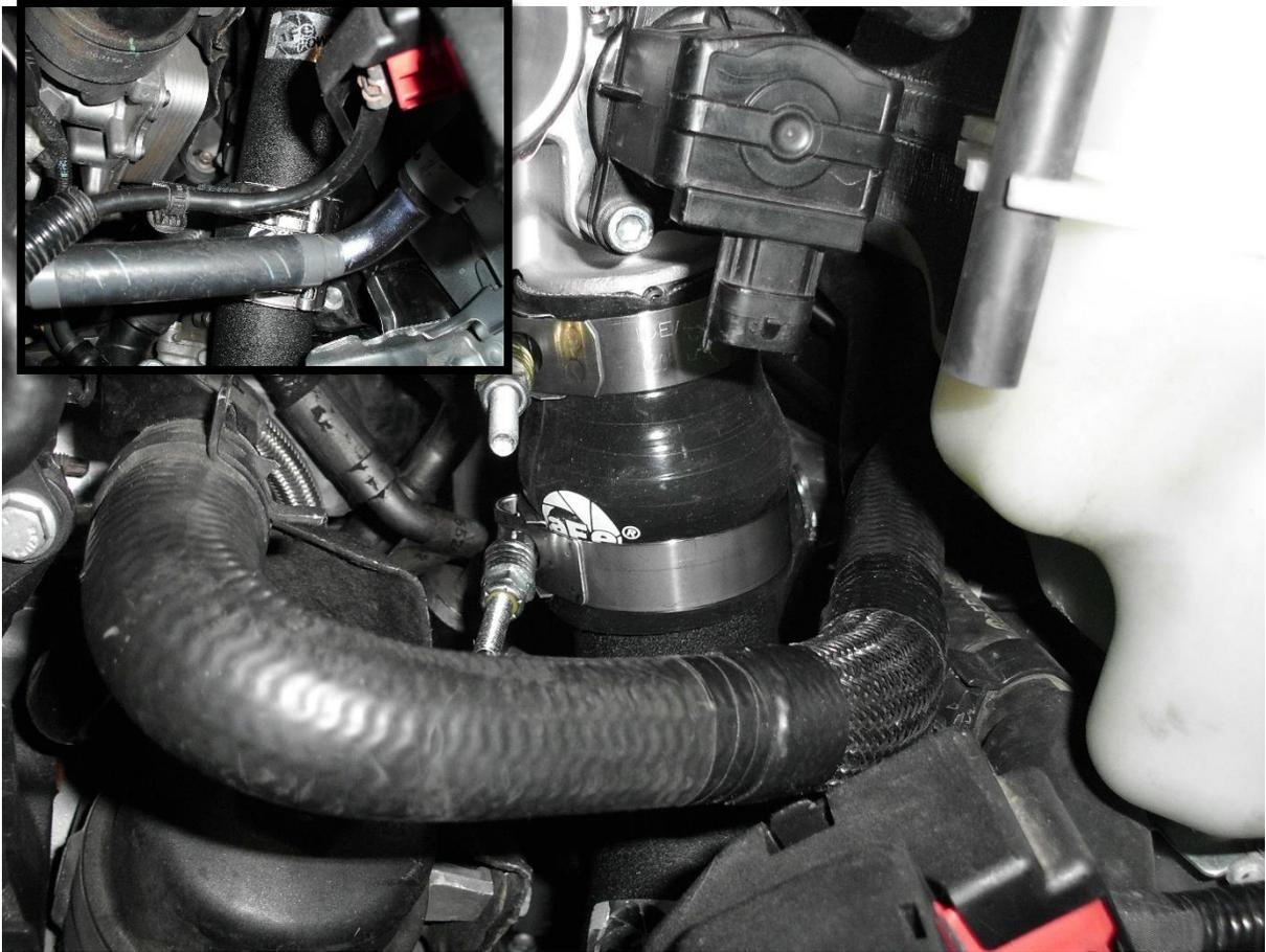
62. Install the supplied 2-1/4" x 1-7/8" coupling along with one (1) of the supplied 2-1/2" clamps onto the end of the aFe upper hot side intercooler tube closer to the fitting (do not tighten the clamp yet).
