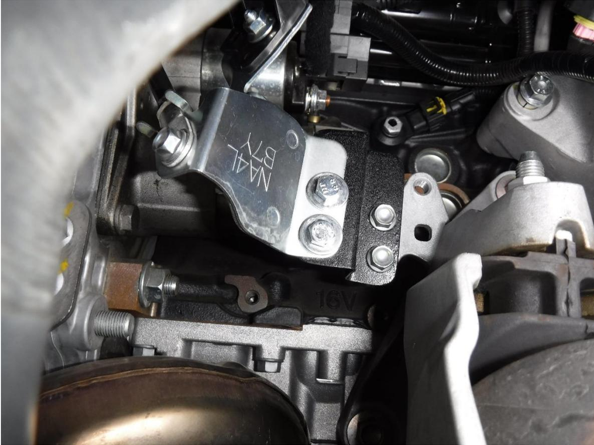
31. Install the supplied aFe wire harness relocation bracket into the vehicle using the factory mounting bolts from step 28 and tighten.
