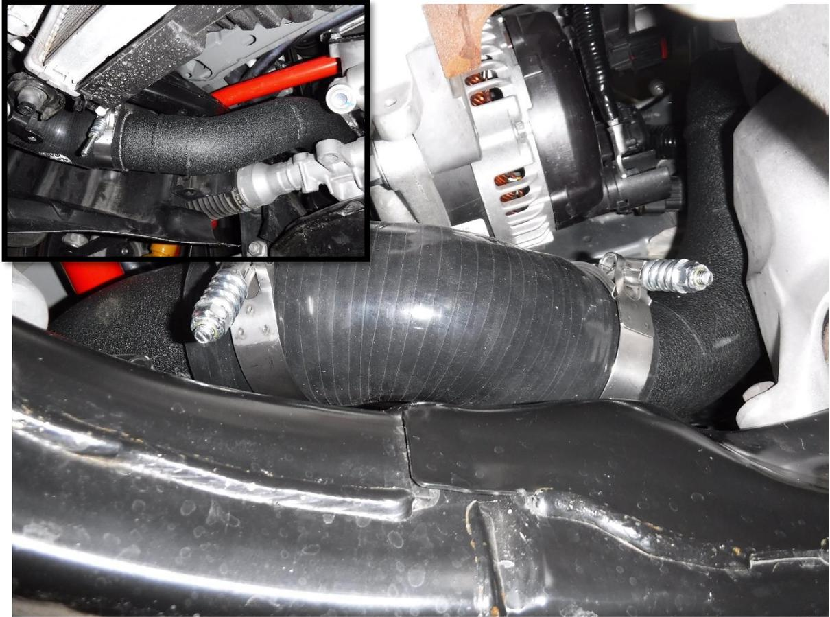
39. Install the supplied 2-1/2" x 45° coupling with one (1) of the supplied 2-7/8" clamps onto the aFe upper cold side intercooler tube.
