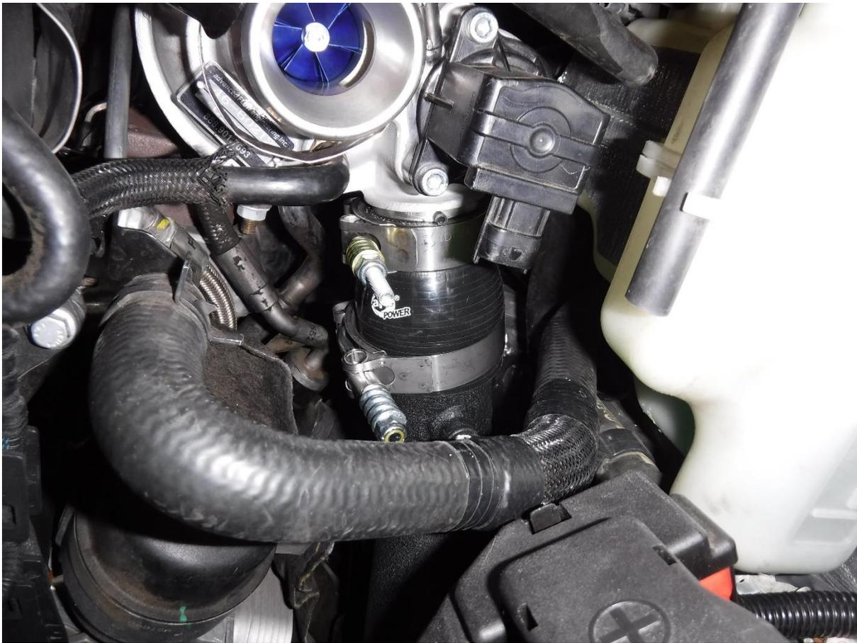
49. Install the supplied 2-1/4" x 1-7/8" coupling along with one (1) of the supplied 2-1/2" clamps onto the end of the aFe upper hot side intercooler tube closer to the fitting (do not tighten the clamp yet).
