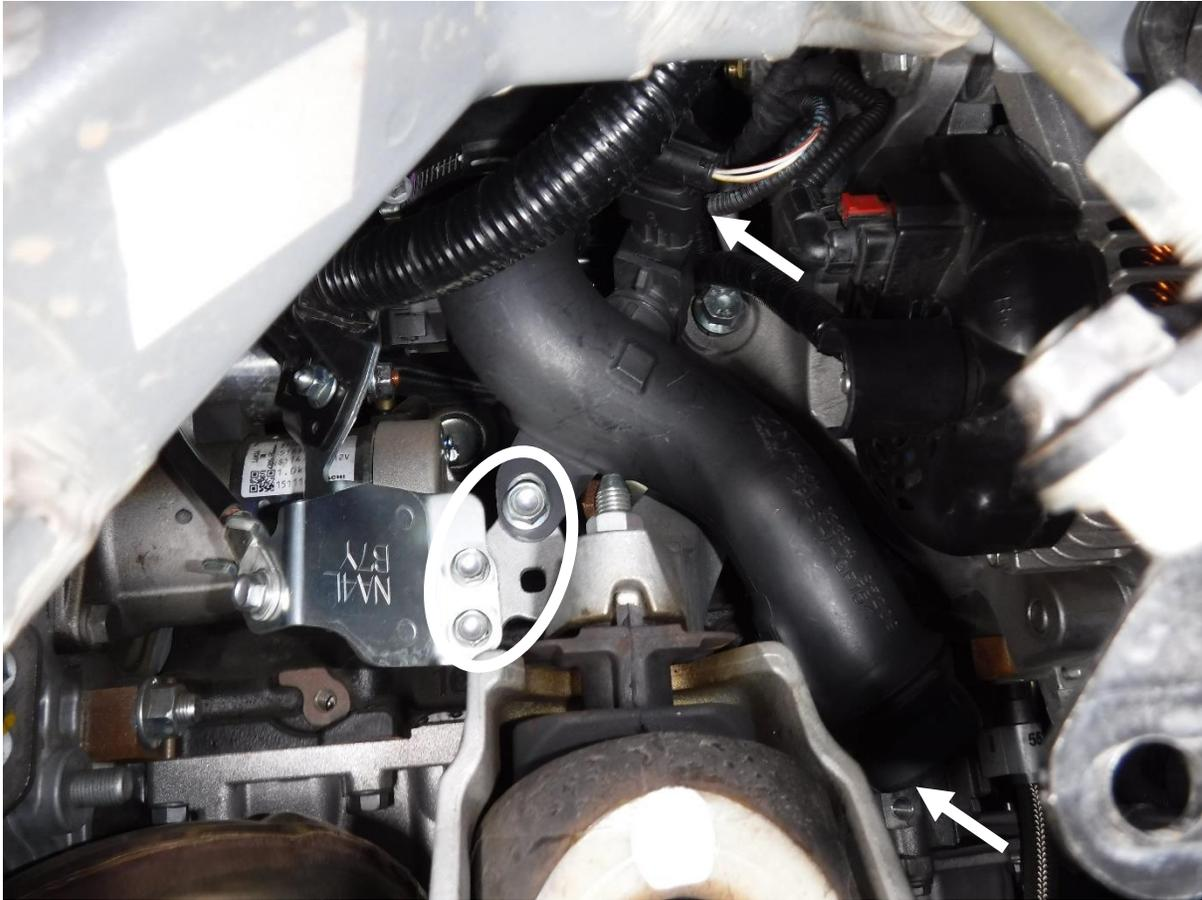
27. Unlock the locking tab on the MAF sensor connection, then disconnect the MAF sensor from the upper cold side intercooler tube.
