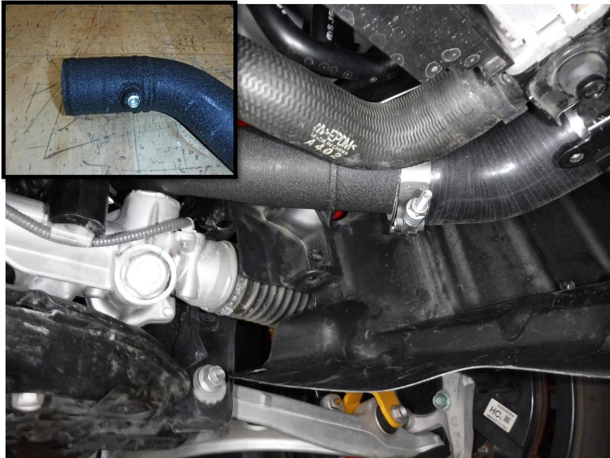
45. Install the remaining 2-1/4" x 1-7/8" x 45° coupling with one (1) of the 2" clamps onto the hot side of the intercooler (do not tighten the clamp yet).
