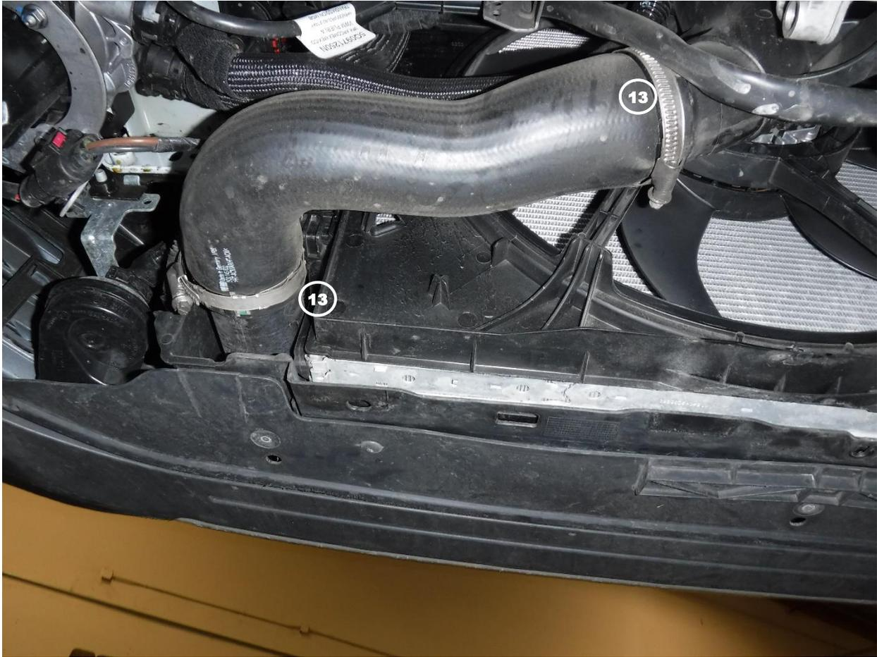
15. Loosen the two (2) clamps securing the lower rubber hot side intercooler hose onto the intercooler and the hot side intercooler tube (13) located on the driver side of the vehicle.
