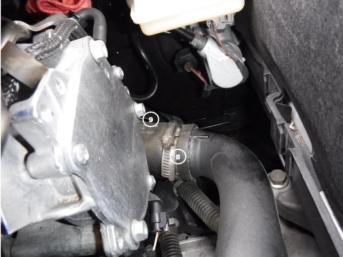
10. Loosen the two (2) clamps securing the hot side intercooler tube onto the turbo outlet (8).
