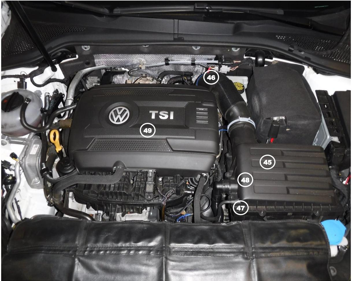
55. Reinstall the air intake scoop into the vehicle.
