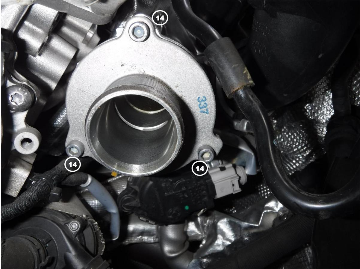
**Note: Be sure not to misplace the O-ring on the back side of the turbo muffler**
