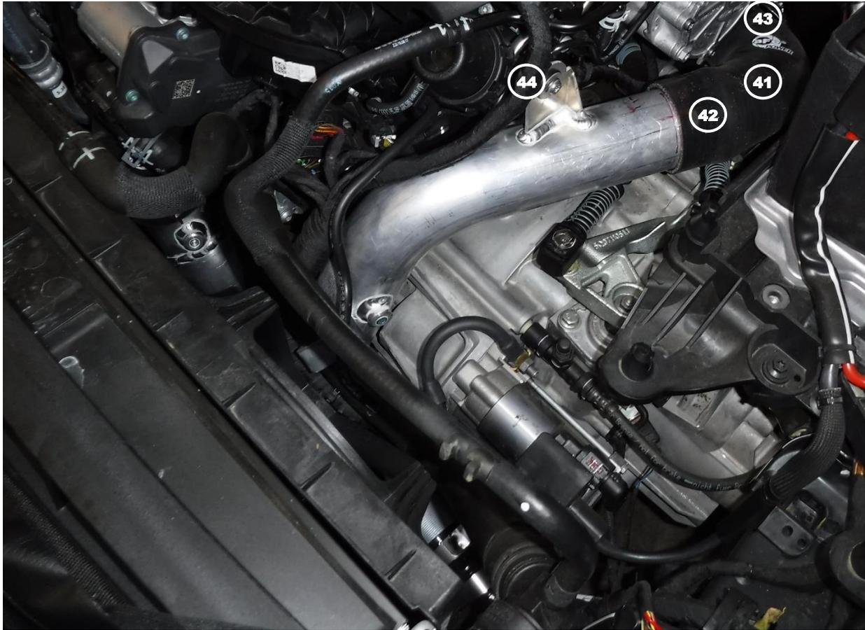
50. Install the aFe silicone turbo outlet coupling, (41) and the remaining 2.85" spring-loaded t-bolt clamp (42) onto the end of the aFe hot side tube, do not tighten the clamp yet.
