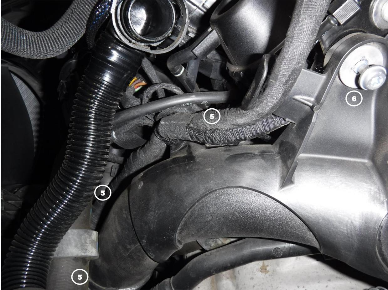
8. Unclip three (3) clips securing the wire harness to the factory hot side intercooler tube (5).
