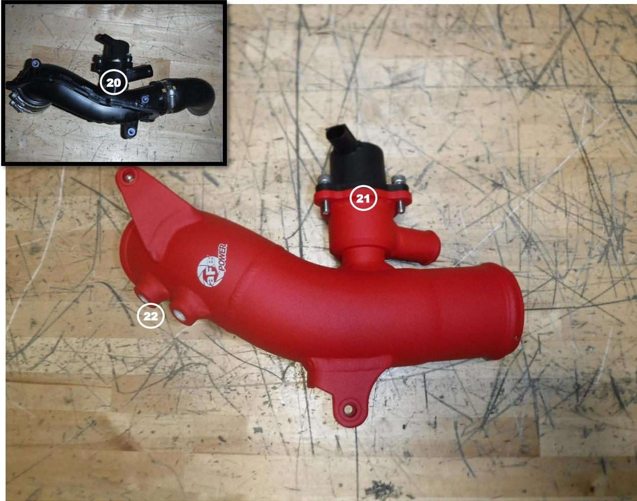
24. Remove the driver's side bypass valve actuator from the factory charge pipe (20)
