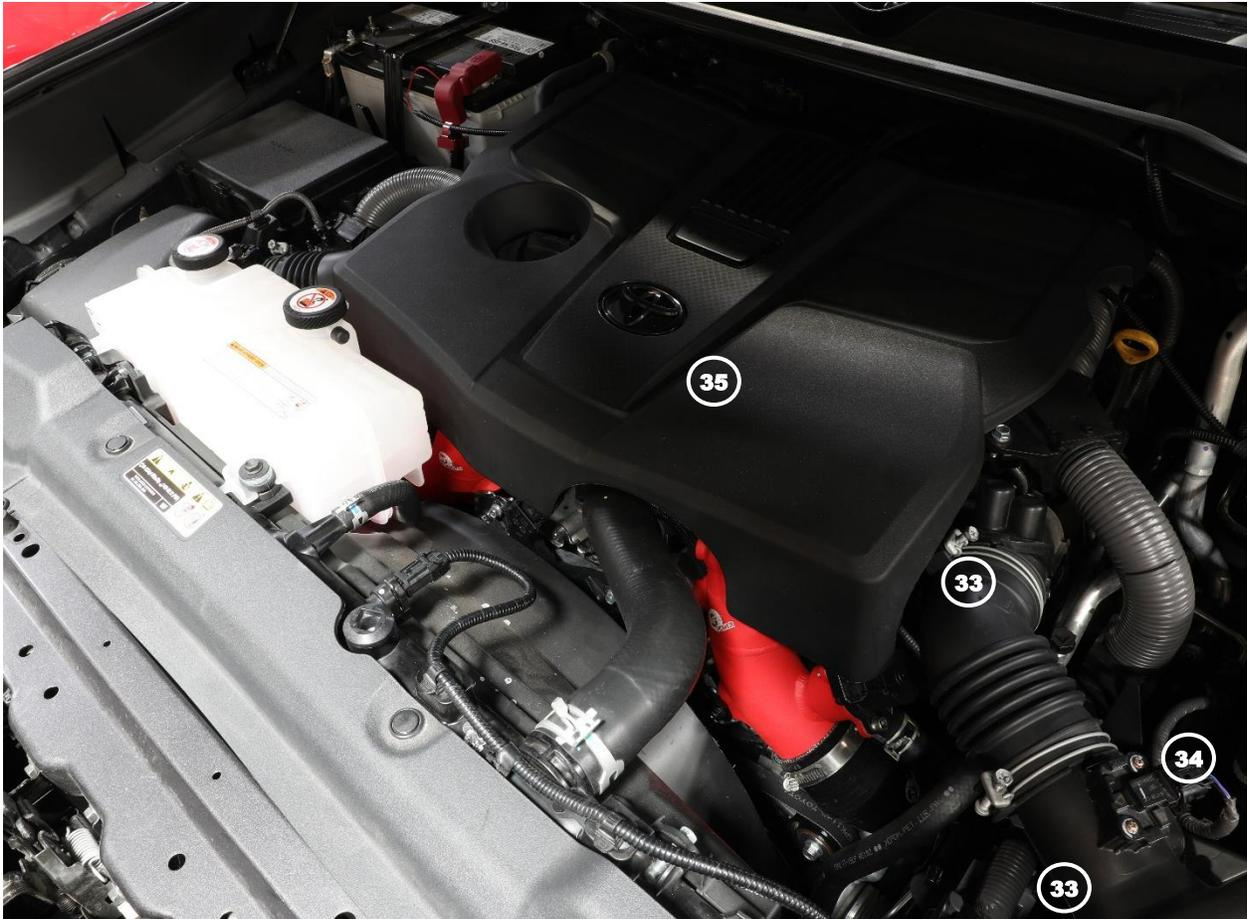
46. Reinstall the air intake tube and air box top into the vehicle and tighten the clamps (33) on both sides.
