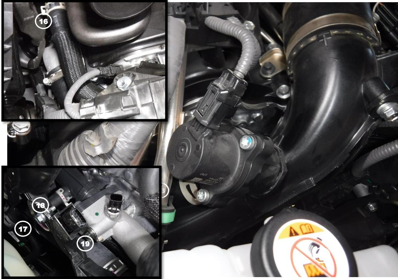
19. Disconnect the bypass valve hose on the passenger side of the vehicle from the turbo inlet tube, located directly above the turbo coupling (16)
