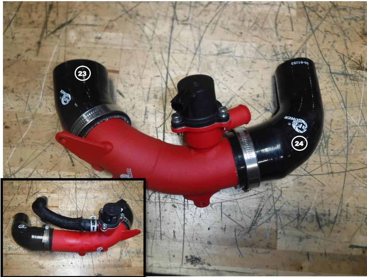
28. Install the supplied 2.5" x 30Deg coupling along with one SmartSeal, 044 (2.50" – 3.06") onto the short end of the aFe charge pipe, ensure that the bead on the inside of the coupling interlocks into the groove on the aFe charge pipe (23)
