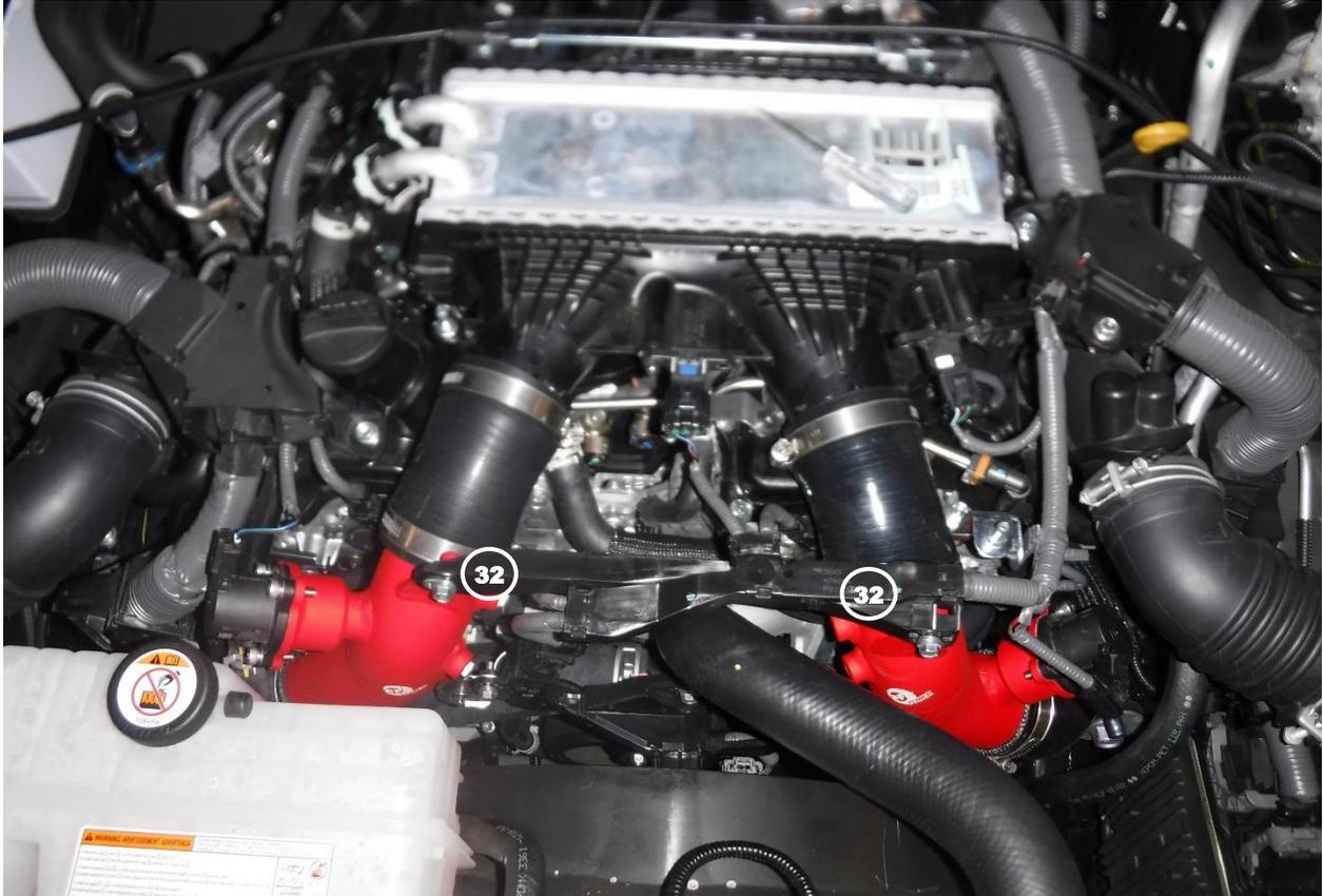
39. Reinstall the factory engine harness mount onto the aFe charge pipes using the factory mounting screws (32) aFe charge pipes will need to be adjusted at this point.
