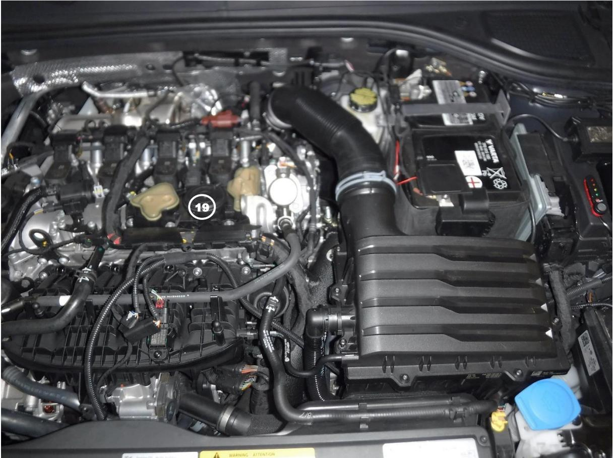
24. Reinstall the engine cover (19) onto the vehicle if equipped.
