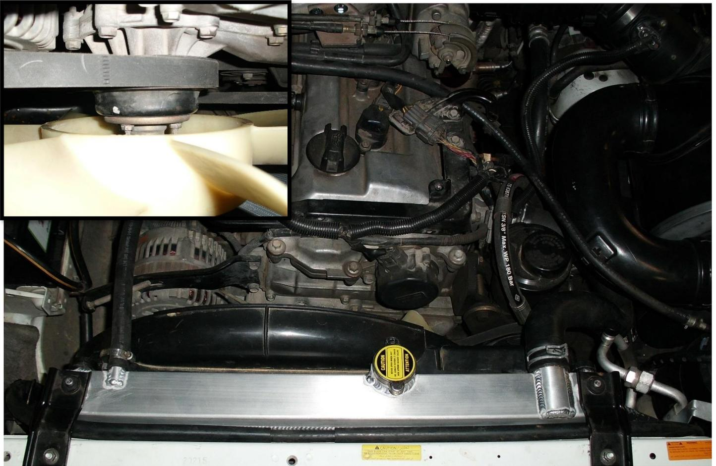
20. Install the aFe radiator into the vehicle, ensuring the side mounts drop into position in the vehicle.
