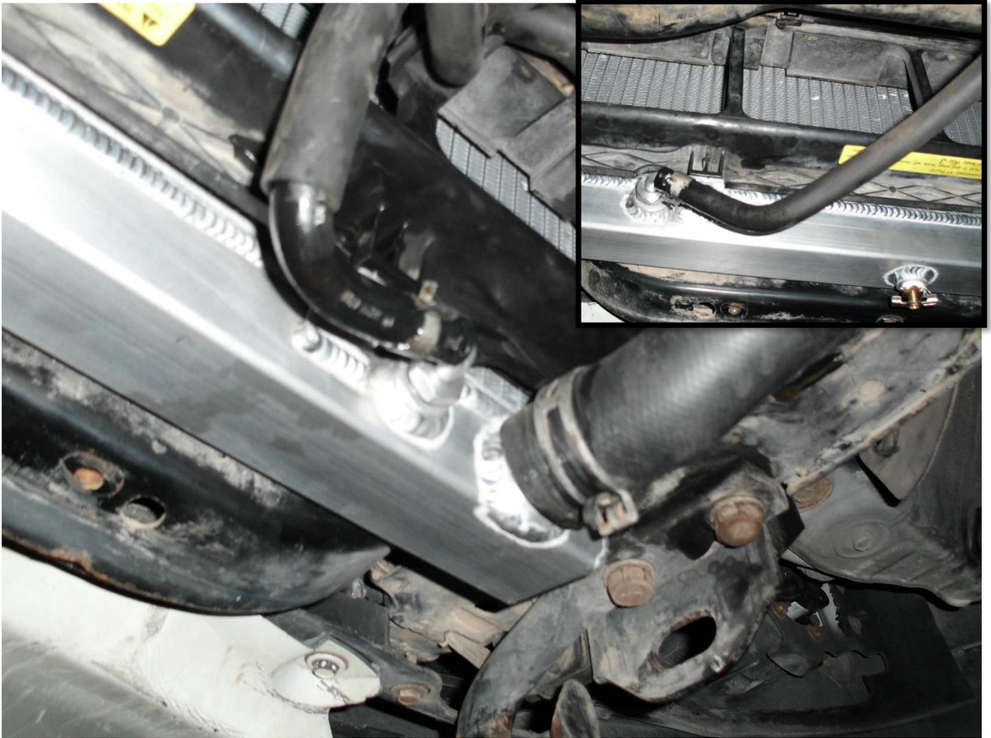
28. Reconnect the lower radiator hose to the radiator and secure with the factory clamp.
