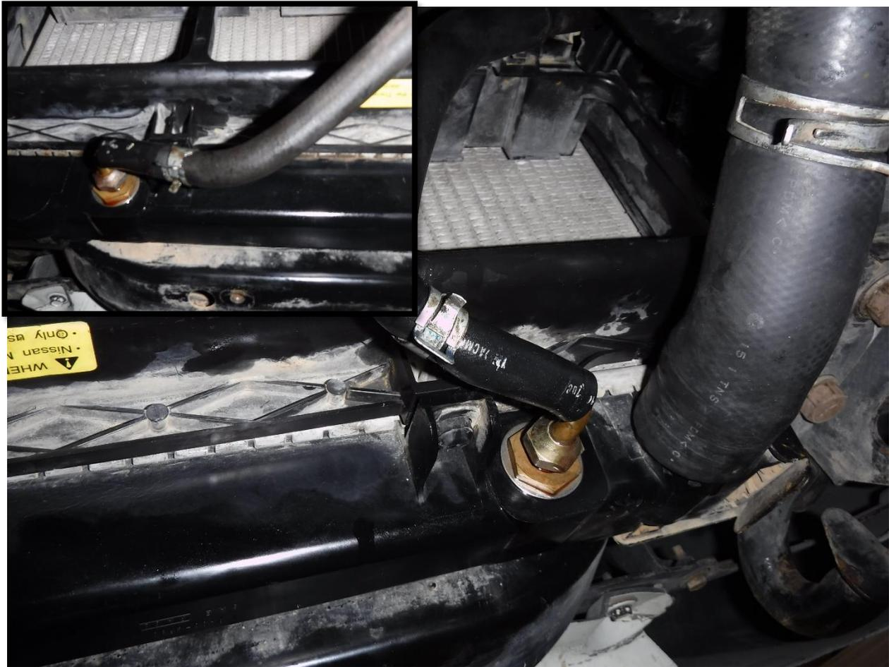
7. Disconnect the lower radiator hose from the radiator.
