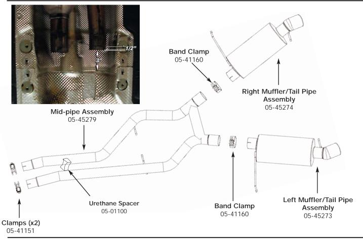
**Step 1:** (Read Instructions prior to installation) Remove your stock exhaust from the rear of your vehicle working your way forward. Take caution not to damage the factory isolation mounts as they will be reused. It is recommended to not fully tighten the clamps until the entire system has been installed.
