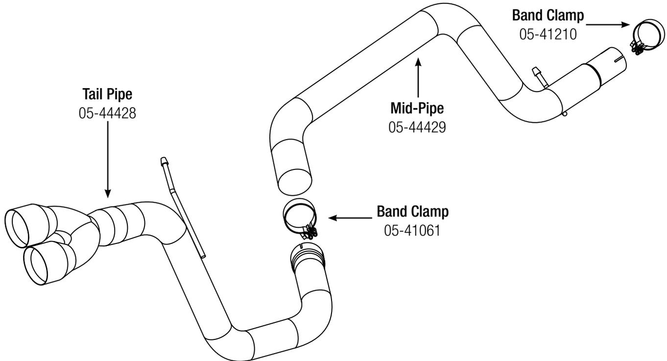
**Step 1: (Read Instructions prior to installation)** Remove your stock exhaust from the rear of your vehicle working your way forward. **It is recommended to not fully tighten the clamps until the entire system has been installed.**
