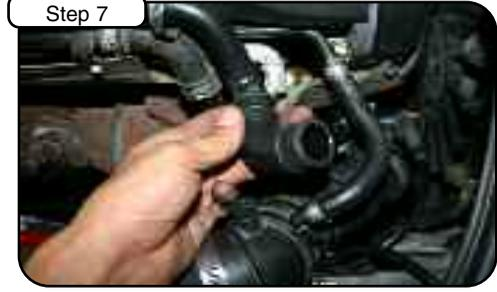
Step 7 Remove clamps holding second breather from top of factory tube. Save elbow for later use.
