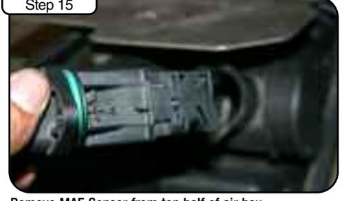
Step 15 Remove MAF Sensor from top half of air box.
