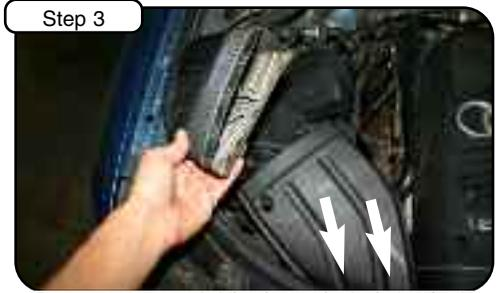
Step 3 a. Remove two screws holding factory fresh air duct in place. b. Pull fresh air duct out of vehicle and save for later use
