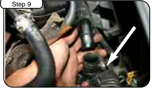
Step 9 Loosen clamp holding fourth breather down from top of tube with slotted screwdriver.
