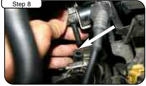
Step 8 Remove clamps holding third breather filter from top of factory tube. Plug can be disconnected for ease of removal.
