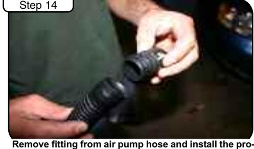
Step 14 Remove fitting from air pump hose and install the provided breather filter. Install the filter onto the air pump and reinstall fog lamp and grill.
