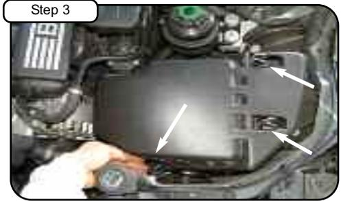
Detach the 3 Factory clips holding in upper half of OE airbox.
