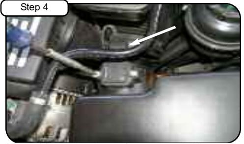
Using 1/4" nut driver, loosen factory clamp holding upper airbox. With T20 torx bit loosen the 2 bolts holding in MAF sensor. Carefully remove MAF sensor from airbox.
