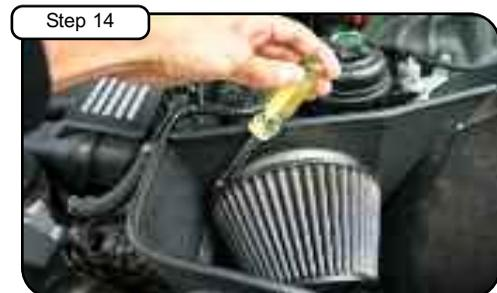
Install your high FLOW air filter. Tighten using 5/16" nut driver.
