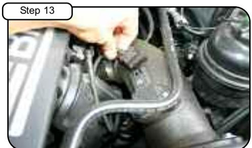
Carefully install MAF sensor into new tube. Place gasket between tube and sensor and tighten with screws provided. Connect MAF sensor harness. Tighten coupler clamps with 5/16" nut driver.
