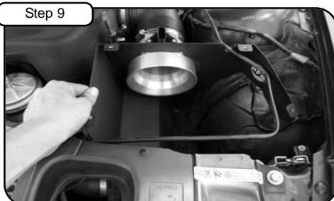
Install housing into vehicle.
