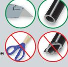
The minimum bend radius for 1/4" air line is 1" (25mm). Air lines are to be installed straight into fittings.
