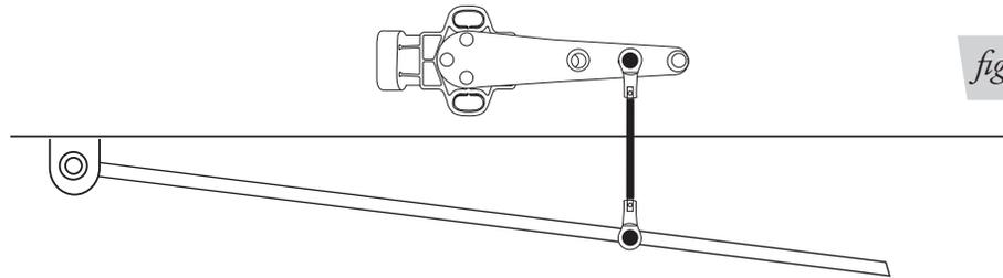
4. Loosen if needed in order to extend to reach the lower mounting point. If loosening the linkage to extend, it is required to make sure to have at least 5 threads of engagement on both ends (fig. 25).
