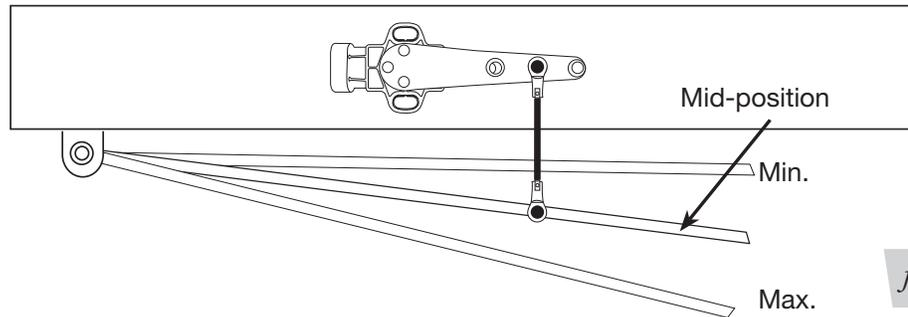
3. Fasten by finger tightening the linkage to the sensor arm and ensure the sensor arm is at mid-position with respect to the sensor (fig. 24).
