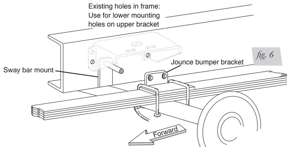
3. Center punch the upper (and, if needed, the lower) mounting holes.
