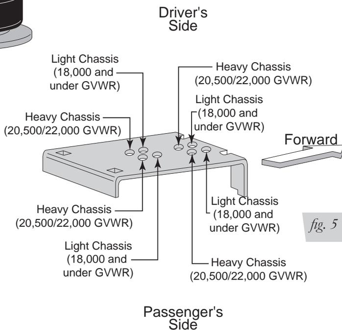
5. Upon determining the correct mounting holes on the lower bracket, insert two carriage bolts (J) into the lower bracket (fig. 1). Attach the air spring assembly to the lower bracket using two 3/8" bolts (F), lock washers (G), and flat washers (H). Tighten bolts to 20 ft/lbs.
