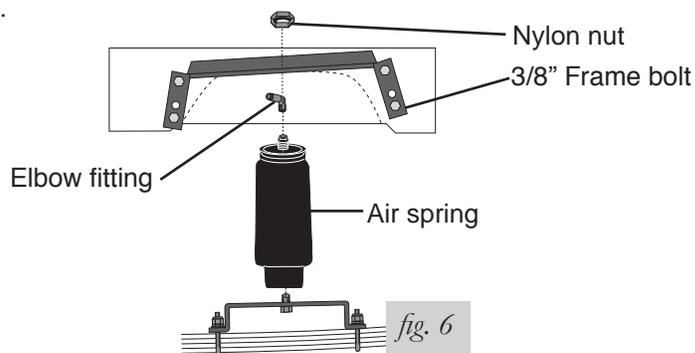
7. Install the elbow fitting into air port of the air sleeve. The fitting is precoated with thread sealant. Tighten finger tight plus two turns. Use a 7/16" open end wrench being careful to tighten on the metal hex nut only. Do not overtighten (fig. 6).
