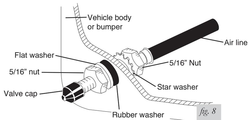
5. Push the inflation valve through the hole and use the rubber washer, flat washer, and another 5/16" nut. Tighten the nuts to secure the assembly in place (fig. 8).
