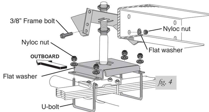
3. Attach the lower bracket as shown in fig. 4 using the u-bolts, flat washers and lock nuts. Tighten nuts to 20 ft/lbs.
