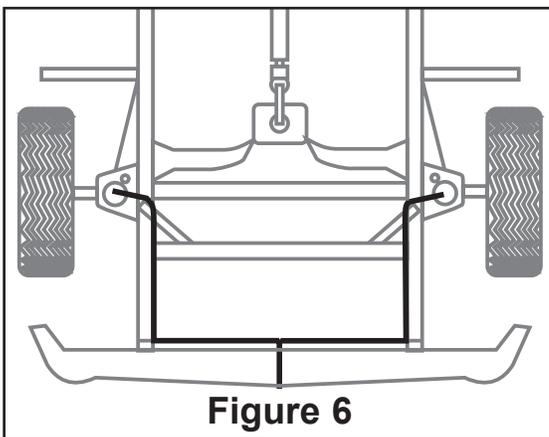
Tee air line installation recommended unless weight in vehicle varies from one side to the other and unequal pressures are needed to level the load. Dual air lines are used in this case.
