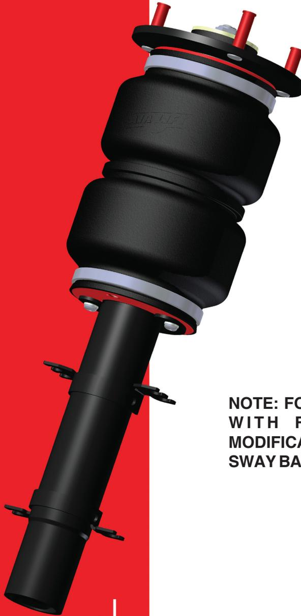
**NOTE: FOR USE ON VEHICLES WITH FRAME C-NOTCH MODIFICATIONS ONLY. FRONT SWAY BAR MUST BE REMOVED.**
