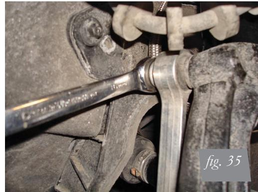
10. Make sure the lower fork/shock mount is fully seated against the shock adapter, install the nut and bolt and torque to 40Nm + 180 degree turn (29.5lb-ft + 180 degree turn) (fig. 36).
