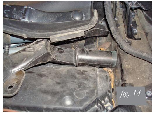
6. Unbolt and remove the washer fluid filler neck with tube (fig. 15).
