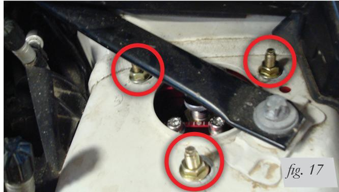
2. The factory strut tower brace needs the provided flat washer placed underneath the outboard attaching point. This will allow the use of the damping adjustment knob. Unbolt (Fig. 18) and place the flat washer under the brace (Figs. 19 & 20), bolt back in (Fig. 21).
