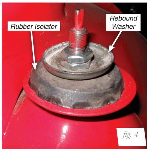
3. Remove the rubber isolator from the shock rod and retain for later use (fig. 5).
