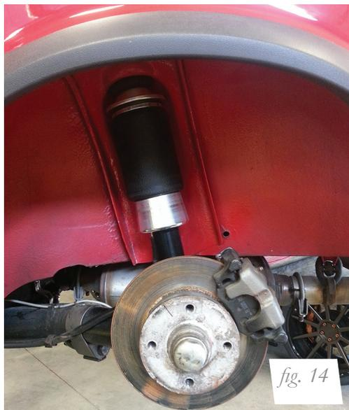
4. Fully compress the suspension using a jack. With the suspension compressed, review the best routing for the leader hose that is clear of all suspension components and axle. Routing should also allow for the suspension to extend without kinking or pulling the line tight or rubbing on other components. Check clearances to all other components.
