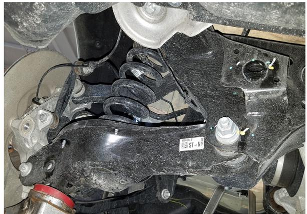
4. Remove ABS wire from shock tab. On vehicles equipped with adaptive suspension, remove the connector from the rear shock (not shown).
