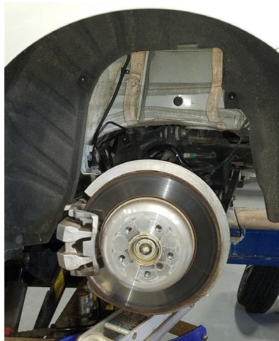
2. Remove lower control arm rock guard. Support lower control arm with jack.
