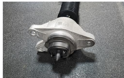
6. Insert upper shock mount into vehicle chassis. Install bolts and torque to 28Nm (20 lb.-ft.).
