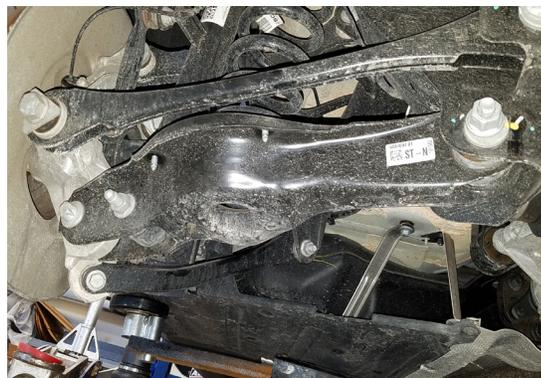
3. Remove inner and outer toe link bolts. Remove toe link from vehicle.
