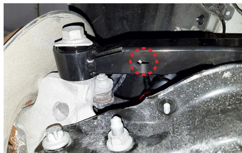
9. Reinstall lower control arm rock guard and torque nuts to 6Nm (4 lb.-ft.).
