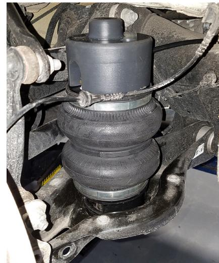
3. Install centering spacer with bolt. Centering spacer offset should have the bolt toward the front of the vehicle. Torque bolt to 30Nm (22 lb.-ft.).
