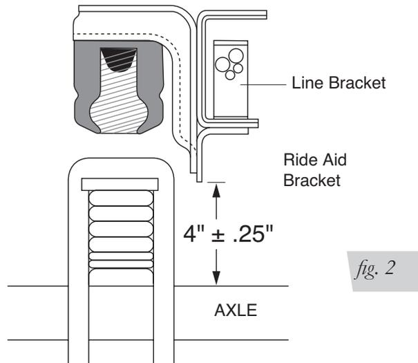
Normal Ride Height is the distance between the bottom edge of the wheel well to the center point of the hub with the vehicle in an “as delivered condition” (without a load, i.e. tool box, camper, etc.). Measurements should be taken before beginning the installation. The distance from the bottom edge of the wheel well to the center point of the hub should be recorded. This kit is designed to be installed and operated at normal ride height.
