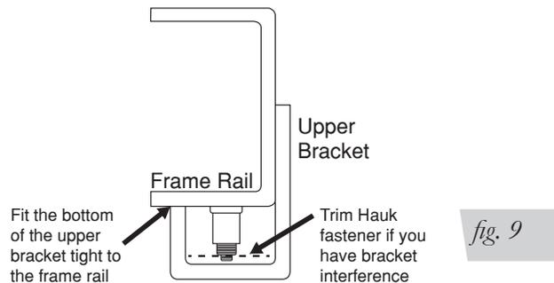
4. Once the upper bracket hardware is tight, adjust the lower bracket forward or back so that the bellows is parallel between them and torque the carriage bolt mounting hardware to 16 lb.-ft. (Fig. 1).
