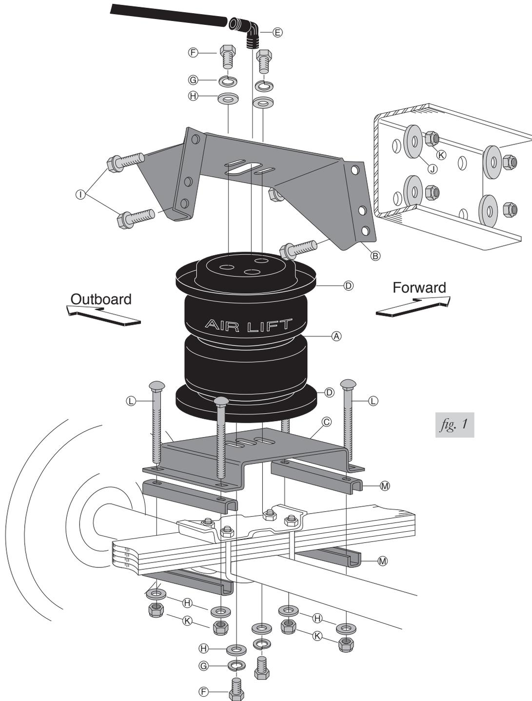
**IMPORTANT:** Check both sides of the frame rail for any interference or obstructions (specifically, propane lines) that may prevent install the air springs on the outside of the frame rail. If obstructions are present, use kit 57131, which mounts under the frame to the axle.
