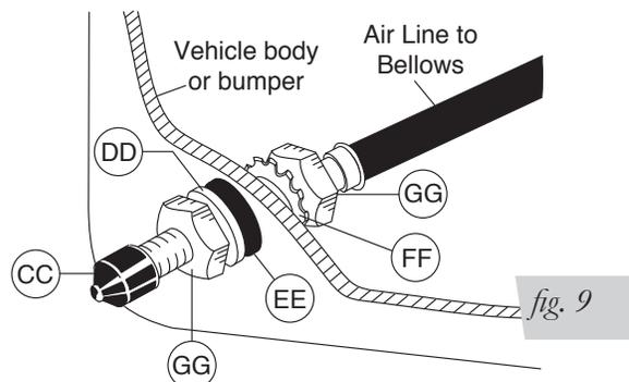
6. Route the air line along the frame to the air fitting on the air spring. Keep at least 6" of clearance between the air line and heat sources, such as the exhaust pipes, muffler, or catalytic converter. Avoid sharp bends and edges. Use the plastic tie straps (BB) to secure the air line to fixed, non-moving points along the chassis. Be sure that the tie straps are tight, but do not pinch the air line (Figure 10).
