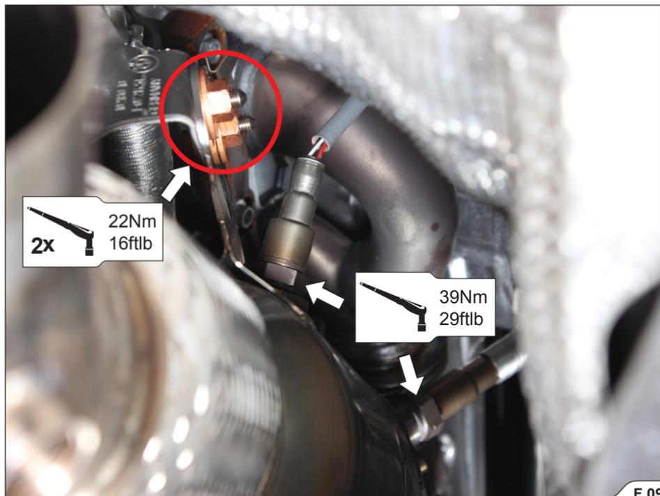
3. Tighten the marked clamp to the specified torque (**F 10**).
