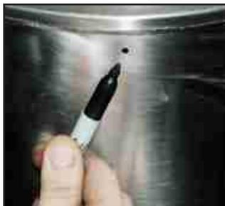
NOTE: IMPORTANT-Make sure that the small drain or weep hole in muffler faces down when muffler is installed.
