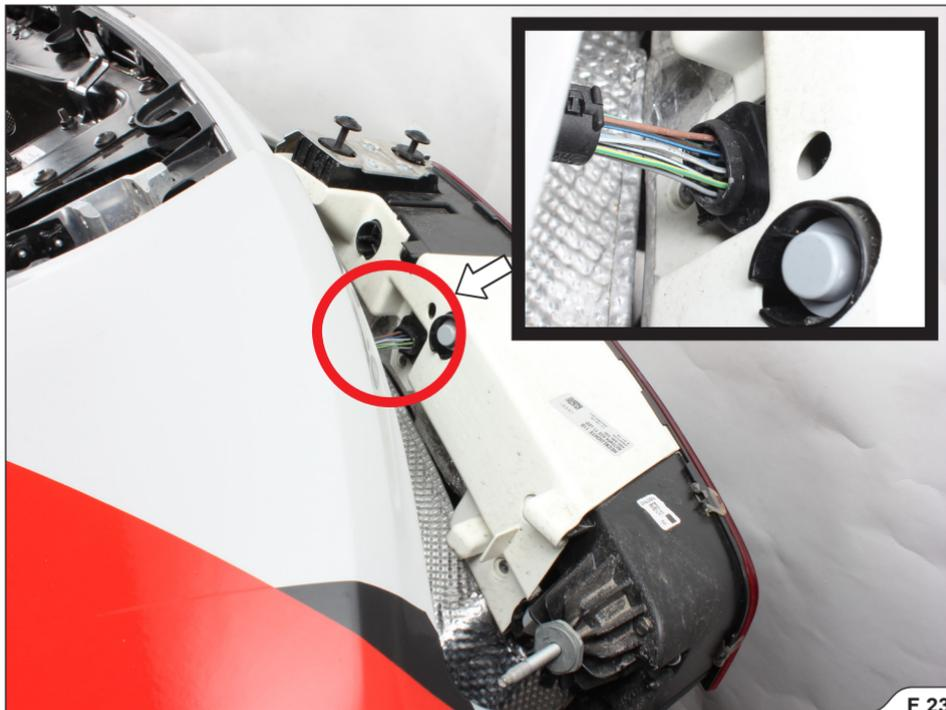
11. Undo and disconnect the number plate's lights, unscrew marked bolts, disconnect the marked connector and carefully remove the lower tail trim panel off the vehicle (F 24, 25).
