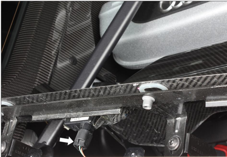
6. Unscrew the marked bolts and carefully remove the muffler panel off the vehicle (F 12, 13, 14).
