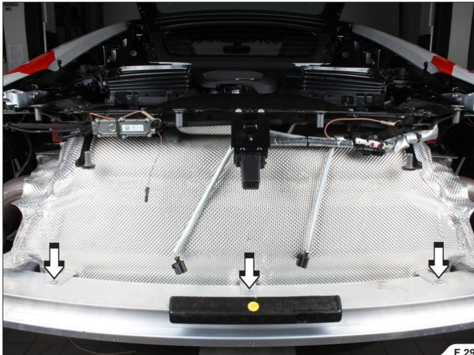
14. Unscrew and remove the bracket and remove the vacuum tubes off the air boxes (F 30).
