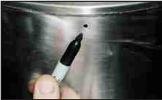
**NOTE: IMPORTANT:** Make sure that the small drain or weep hole in muffler faces down when muffler is installed.
