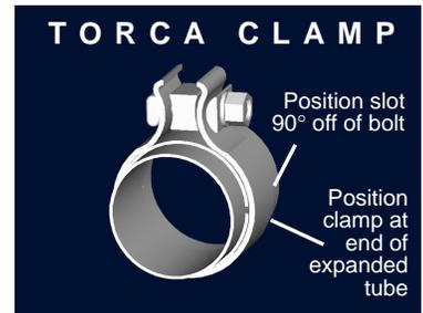
8. It is mandatory that all clamps be checked and tightened if necessary after road testing the vehicle once the system has cooled.
