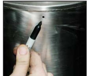
**NOTE: IMPORTANT:** Make sure that small drain holes in rear of each tunnel muffler face down when installed.
