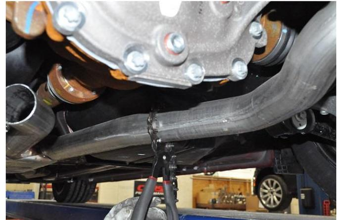
**4.** Using a chain cutter or similar device, cut both the driver and passenger side exhaust pipes at the marked locations. Place an adjustable stand or similar device under the stock tunnel section of the exhaust for support. Once the axle pipes are cut, there are no additional stock hangers supporting the tunnel section.
