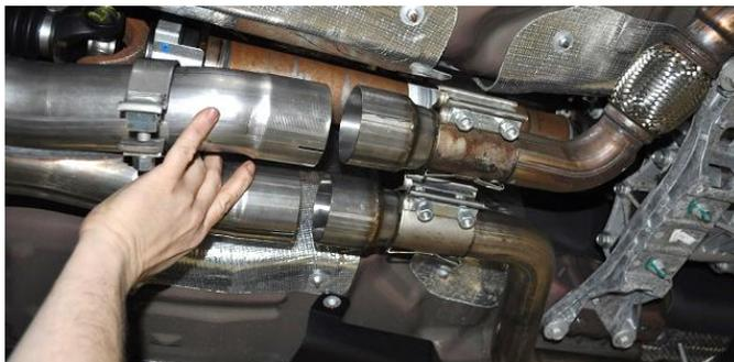
3. Slide the X-Pipe inlets over the X-Pipe adapter outlets.
