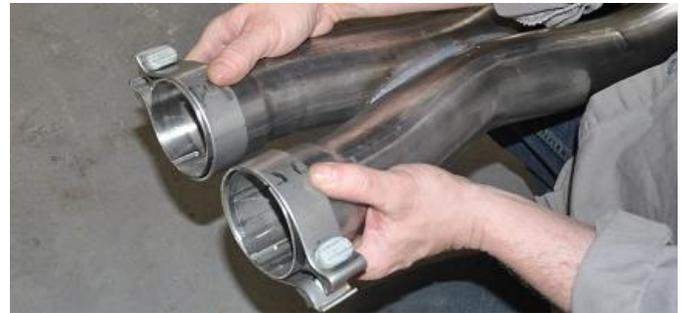
2. Install two 3" clamps on the driver and passenger inlets of the Double X-Pipe so that the bolts are vertical with the nut towards the ground and the bolts towards the outside of the vehicle.
