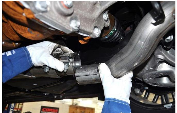
8. Slide the muffler inlet pipe into the driver side adapter outlet. **NOTE:** The use of a soap and water solution may aid in the installation of hanger grommets
