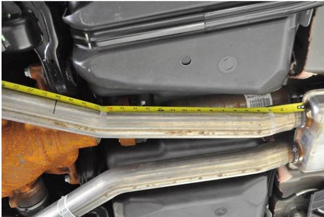
**3.** On the passenger side, measure 23" away from the flange on the stock resonator following the outside profile of the exhaust pipe. Again, the tape measure should follow the bend profile of the pipe.
