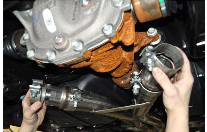
6. Locate two 2 1/2" clamps. Install the clamps on the adapter outlet pipes so that the bolts are vertical with the nuts towards the ground and the bolts towards the outside of the vehicle. **WARNING:** Do NOT tighten the clamps at this step, as the stock axle pipes will then not be able to fit inside the adapters.
