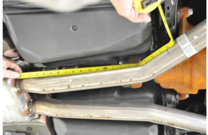
**2.** The tape measure should follow the bend profile of the pipe.
