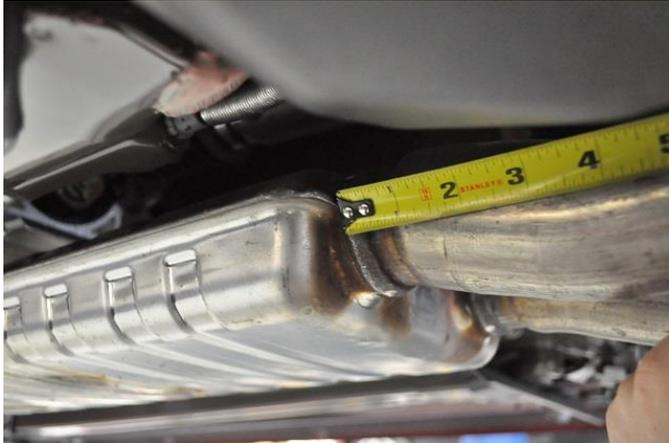
**1.** Starting on the driver side, measure 22½" away from the flange on the stock resonator, following the outside profile of the exhaust pipe.
