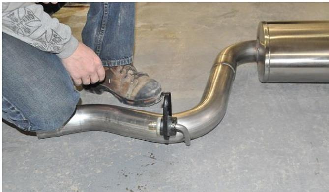
2. Locate the passenger side hanger grommet assembly removed during **Removal Step 7** of the stock exhaust removal process along with the passenger side muffler assembly. Install the hanger grommet assembly onto the front hanger of the muffler assembly in the same position as previously installed on the stock exhaust.
