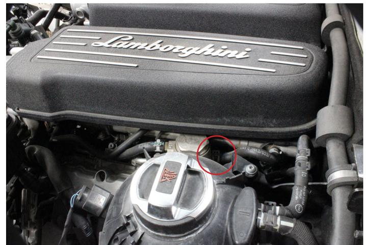
6. Disconnect the 2 connectors on the backside of the manifold near the firewall and the two throttle body connectors. We have shown a manifold off the car to help locate exactly where they are.
