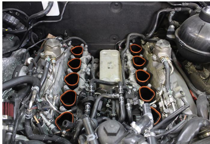
9. Install the intake runner gasket retainers on each runner. The notch on the underside will fit into the groove on the lower intake manifold runners.
