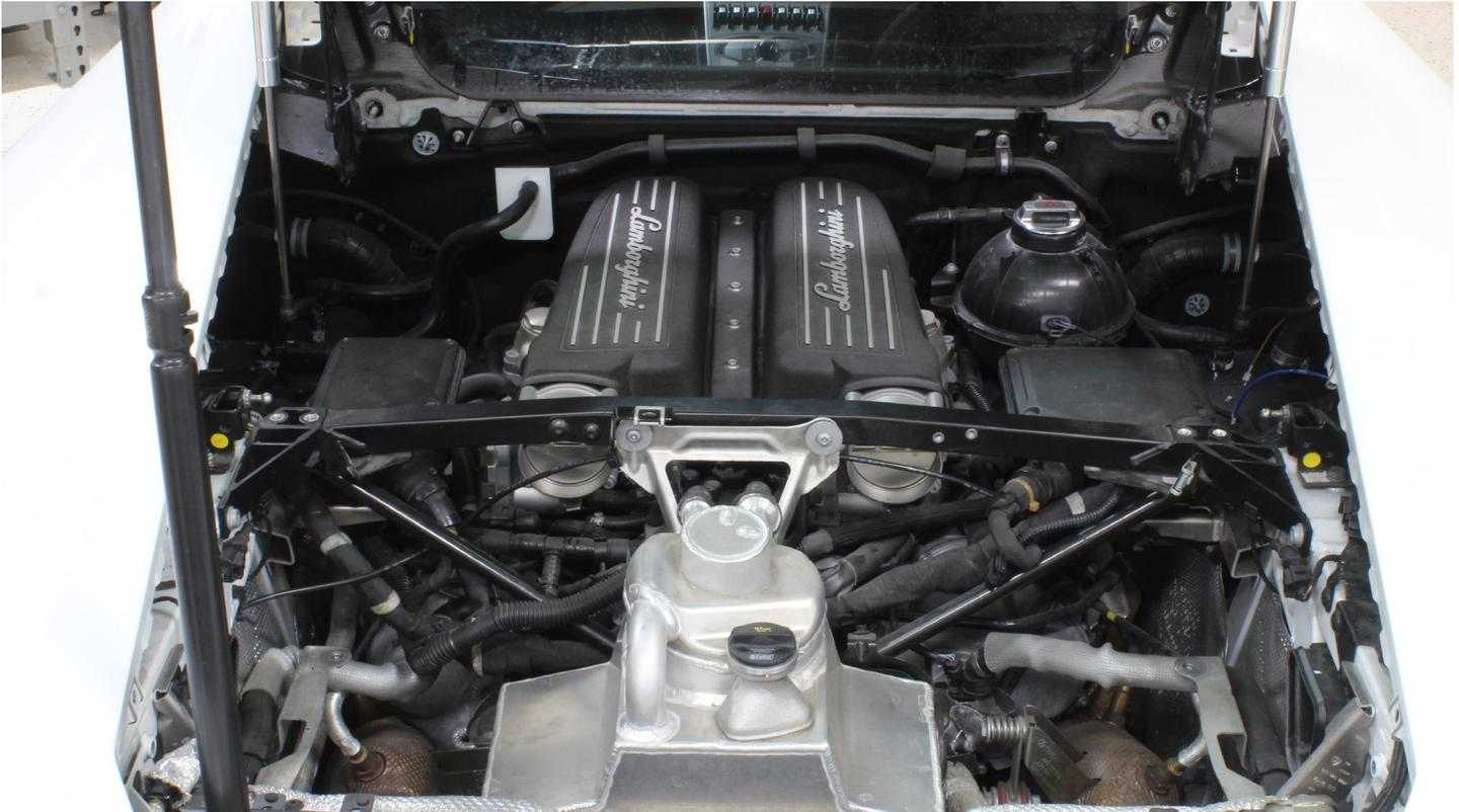
5. Disconnect fuel line on both sides of the manifold and remove bolts holding the hose bracket. Once the bracket is removed you will notice a pressure sensor, disconnect this also.
