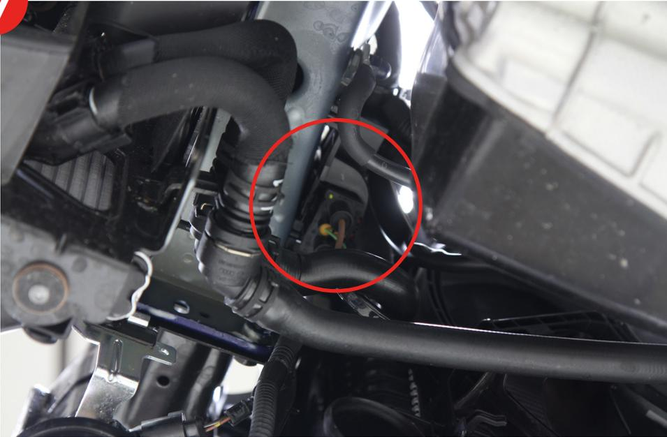
18. Disconnect the outside air temperature sensor. Pull the harness out of its holding clips and pull back to the side.
