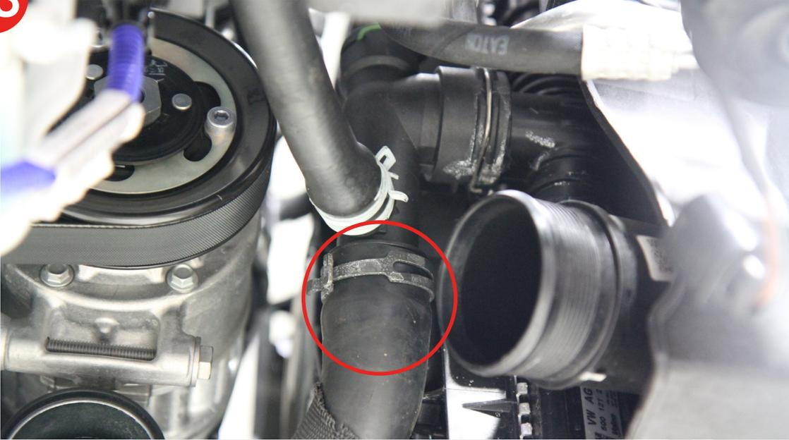
24. When the coolant is drained, reinstall the radiator hose. Disconnect both main radiator hose connections at the radiator quick connects by sliding out the metal retaining clip.
