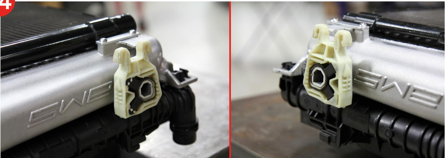
35. Reinstall the cooler assembly back into the core support making sure the retaining clips fully seat into place. Then reinstall the core support back into the car. Make sure to align the core support up with the original mounting bolt locations.
