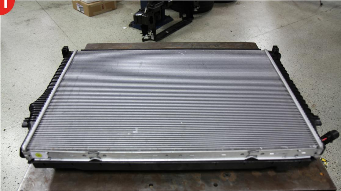
32. Install the AMS intercooler in the reverse order making sure the upper mounting clips are fully seated.
