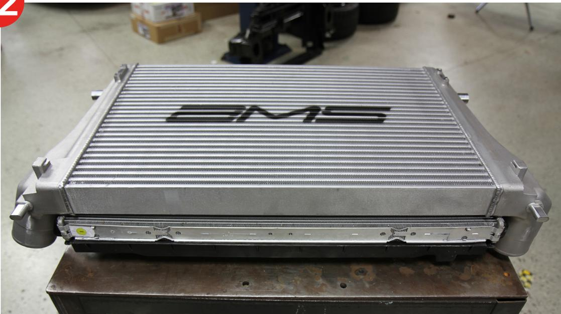
33. Reinstall the A/C condenser on to the intercooler. Locate the two retaining plates and four M5 button head bolts. Install the retaining plates and hardware to the upper A/C condenser mounts.
