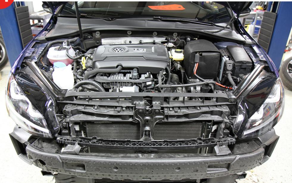
**15.** Remove both front head lights. When removing the headlights, make notes of how everything is adjusted. Each bolt has adjustments and making notes here will aid in reassembly. Follow the next several steps.
