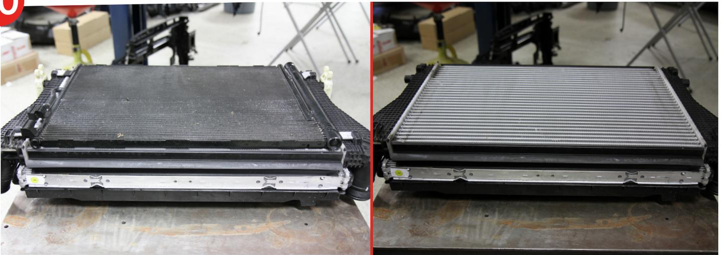
31. Next remove the intercooler from the radiator. Release the clips on the top and pull upward slightly away from the radiator. Next, slide the intercooler downwards off the radiator.
