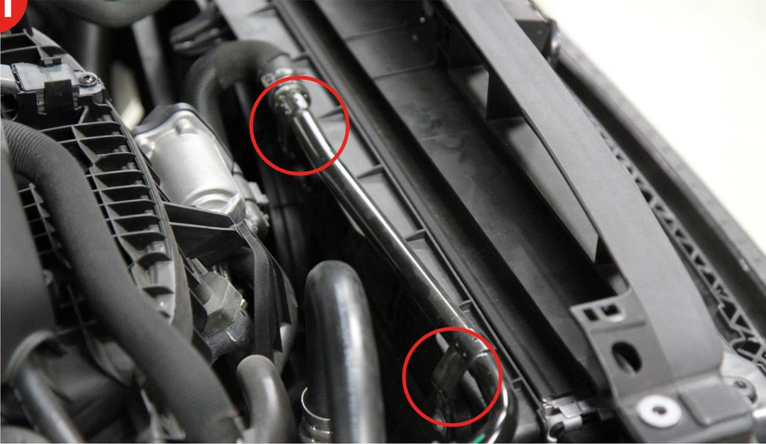
22. Disconnect both horn connectors and harnesses. The horns can remain bolted into place.
