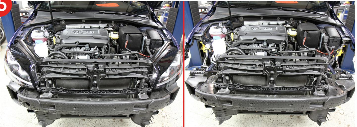
**16.** Remove both factory intercooler hoses. These will not be reused.
