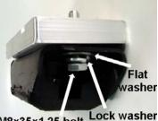
M8x35x1.25 bolt Lock washer S4 Mount Configuration
