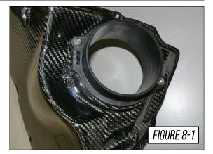
Install the AWE S-FLO Filter onto the AWE Carbon Air Box Lid using the same hardware that attached it to the OE air box lid.
