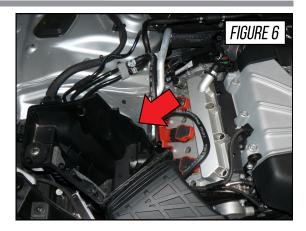
Release the two metal clips holding the MAF housing to the lid. Next, using a T15 Torx bit, remove the two screws securing the air filter element to the lid.
