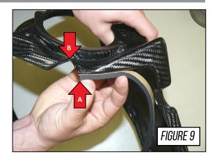
Locate the factory snow shield on the bottom section of the factory air box.
