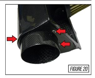
Finish assembling the AWE S-FLO air box by lining up the front and back of the box and bolting it together with the supplied M5X.8 bolts.
