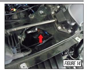
Remove the sound symposer, at arrow in **Figure 15**, from the back of the air box on the driver side by pressing down on its clip and pulling it straight out of the air box.
