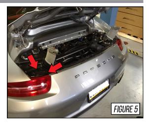
Unclip the wiring connector from the back of the taillights before setting them aside.
