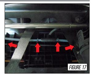
Pull straight up on the air box to release its two mounts from their rubber grommets.
