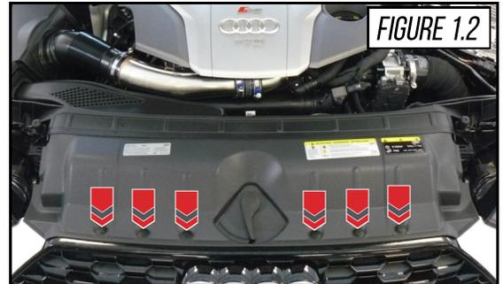
Remove the upper radiator cover by lifting up at the arrows in **Figure 1.3**. Lift and slide forward to remove the cover completely.
