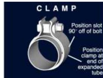
**NOTE:** Align all clamps so that the center of the clamp bolt is 90 degrees from the notch in the pipe. (See Fig. CLAMP)
