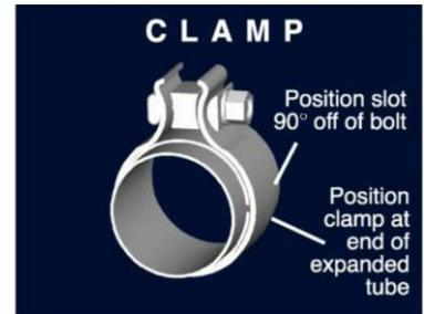
1. Locate the driver side ("**D**" etch) and passenger side ("**P**" etch) clamp on elbow assemblies, along with the driver and passenger side trimmed factory axle pipes retained from the last step in the removal process.
