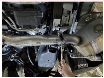
Snugly tighten the clamp securing the muffler inlet pipe using a 15mm deep socket and 3/8" ratchet, leaving it loose enough for later adjustment.
