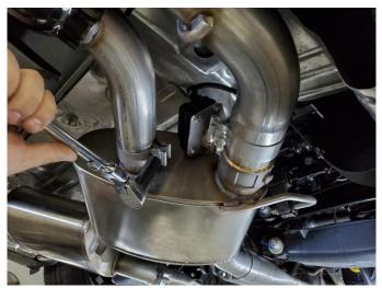
22. Snugly tighten the clamp securing the inner tip assembly to the muffler using a 15mm deep socket and 3/8" ratchet, leaving it loose enough for later adjustment. Repeat steps 19-22 for the driver side inner tip assembly.
