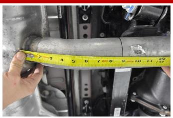
2. Measure 8 3/4" away from the rear muffler case along the underside of the pipe towards the front of the vehicle. Scribe the pipe with a marker at the measured point to create a cut line.
