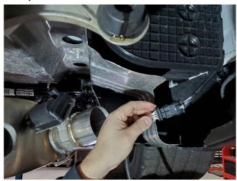
Connect the extension to the stock wiring harness. Press down gray locking tab to secure.
