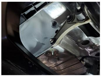
17. Locate the stock hanger grommet assembly mounting hardware from removal step 4 and start them by hand onto the mounting studs.
