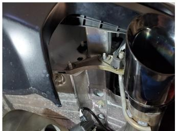
**15.** Install the stock hanger grommet assembly onto the mounting studs.
