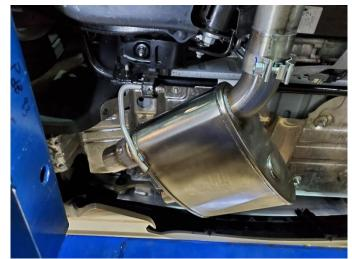
**6.** Slide the inlet pipe over the outlet pipe of the stock exhaust.
