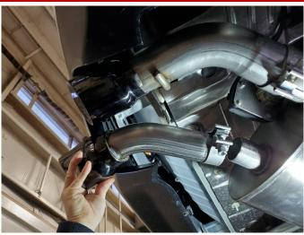
**20.** Slide the tip assembly onto the smaller outlet of the muffler.
