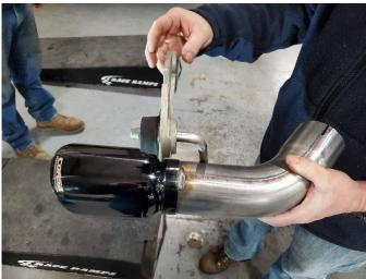
**13.** Install the stock hanger grommet assembly onto the tip hanger.
