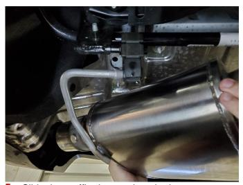
Slide the muffler hanger into the hanger grommet 6. located behind the rear suspension of the vehicle.
