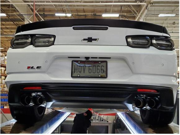
23. Adjust the system accordingly, including the rear muffler rotation and overlap onto the stock exhaust, along with the tip depth and rotation, so that the tips are centered in the bumper valence. Check the position of all hangers to make sure they are properly seated within their corresponding grommets. Check clearances between the system components and chassis. Tighten all clamps to 45ft-lbs using the torque wrench and 15mm socket.
