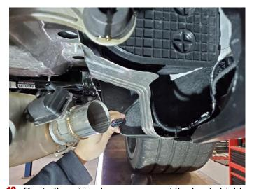
**10.** Route the wiring harness around the heat shield.
