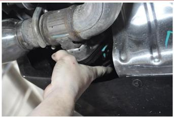
Disconnect the driver and passenger rear NPP (non-AFM) valve plugs located near each of the outer stock exhaust tips.
