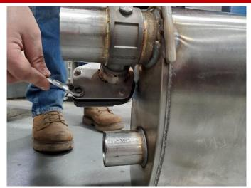
**3.** Tighten the three screws using an 8mm socket and ½" ratchet. Repeat steps 1-3 for driver side muffler.
