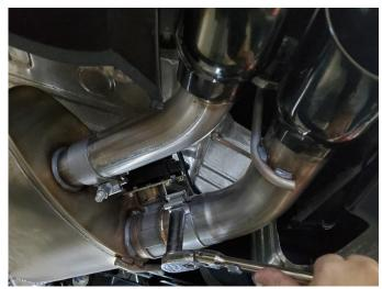
21. Snugly tighten the clamp securing the outer tip assembly to the muffler using a 15mm deep socket and 3/8" ratchet, leaving it loose enough for later adjustment.
