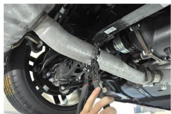
3. Repeat this measurement on the driver side pipe. Using a chain cutter or similar device, cut both the driver and passenger side exhaust pipes at the marked locations. Support the stock rear muffler using a jack stand or similar device.
