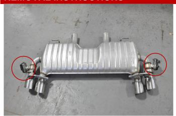
**9.** Remove the three screws securing each valve control unit to the outer stock tips using an 8mm socket and ½" ratchet. Label each unit with the position it was installed to make sure it goes back to the same location.
