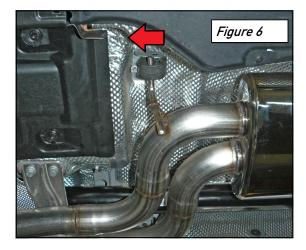
With the slip joint clamps loose, adjust the rear outlet tube assemblies so that the tailpipe outlets are level left to right and are centered in the bumper valance openings. Rotate the outlet tube assemblies to correct for this angle and adjust their slip joints to correct for centering. Once lined up and there is proper clearance around the rear differential and swaybar, as shown at arrow in **Figure 7**, tighten the clamps.
