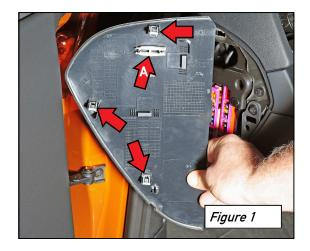
Pop off the purple fuse guard frame on the proper fuse block. Remove the proper fuse as listed in your Owner's Manual. Reassemble fuse block and cover.
