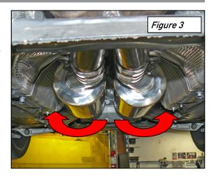
Next install the mid-muffler section, re-using the factory sleeve clamps, making sure the muffler inlets/outlets are sitting level to the bottom of the car.
