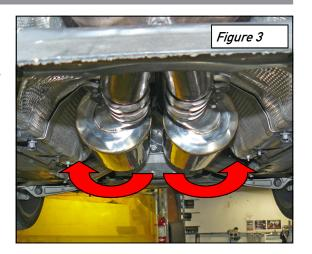
Next install the mid-muf4er section, re-using the factory sleeve clamps, making sure the muf4er inlets/outlets are sitting level to the bottom of the car.
