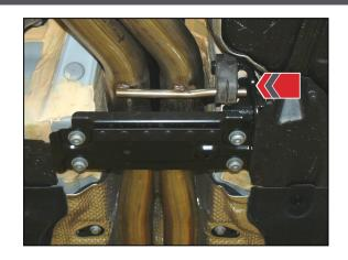
Reinstall the cross brace with the 4 included brace spacers placed between the chassis and the brace, as shown by the arrows in Figure 9.
