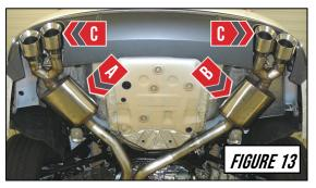
Once the exhaust tips are properly aligned, starting at the downpipe sections moving towards the rear of the car, torque each Accu-Seal clamp to a minimum of 40ft/lbs.
