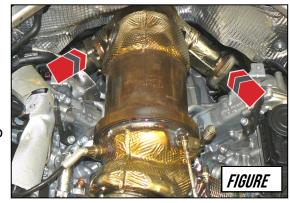
Start by removing the two (2) 12mm nuts on the driver side flange along with the three (3) 12mm nuts on the passenger side flange, as shown by the arrows in **Figure 1**. Five (5) nuts in total can be accessed from the engine bay.
