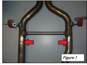
Porsche sleeve clamp, part number 958 111 220 20, can be used to re-attach the balance of the factory system to the front resonator section if the vehicle ever needs to be reverted to stock.
